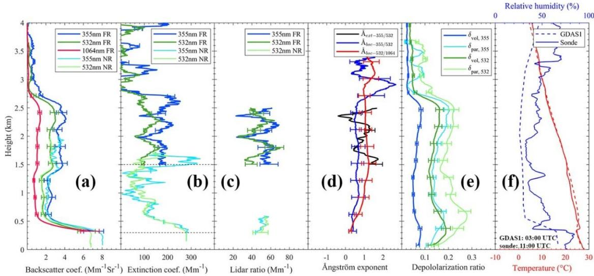
**Figure 8.** Raman lidar observation on 26 November 2018, 02:00-03:00 UTC. (a) Particle backscatter coefficients, (b) particle extinction coefficients (Raman lidar method), (c) lidar ratio, (d) Ångström exponents computed from different wavelengths pair in (a) and (b), (e) volume ( $\delta_{\text{vol}}$ ) and particle ( $\delta_{\text{par}}$ ) depolarization ratios, and (f) relative humidity (blue) and temperature (red) from radiosonde observations and GDAS1 dataset.
