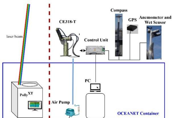
**Figure 3.** Sketch of the Polly<sup>XT</sup> lidar (left of the dashed line) and the shipborne CE318-T (right of the dashed line).
