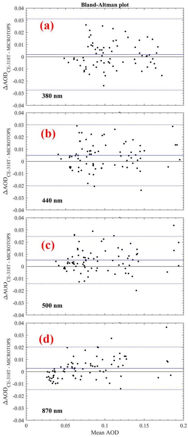
**Figure 5.** Bland-Altman plots for AOD differences with mean AOD  $((AOD_{CE-318T} + AOD_{MICROTOPS})/2)$  at 380 (a), 440 (b), 500 (c) and 870 nm (d). Solid line (black) represents the 0 line. Solid line (blue) represents the mean AOD differences and dotted lines (blue) represent the mean AOD plus/minus the root-mean-squared AOD differences.
