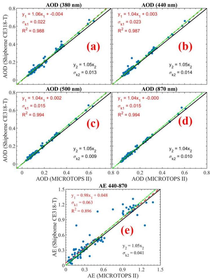
**Figure 4.** Linear regression of AOD (a, b, c, d) and Ångström exponent (e) from the shipborne CE318-T and MICROTOPS II observations. The data points are the mean values within a sliding window of 20 min. 115 data pairs are used in this regression. The red dashed line is the regression result with free intercept relationship and the green dot-dashed line represents the regression relationship with forced intercept through 0.
