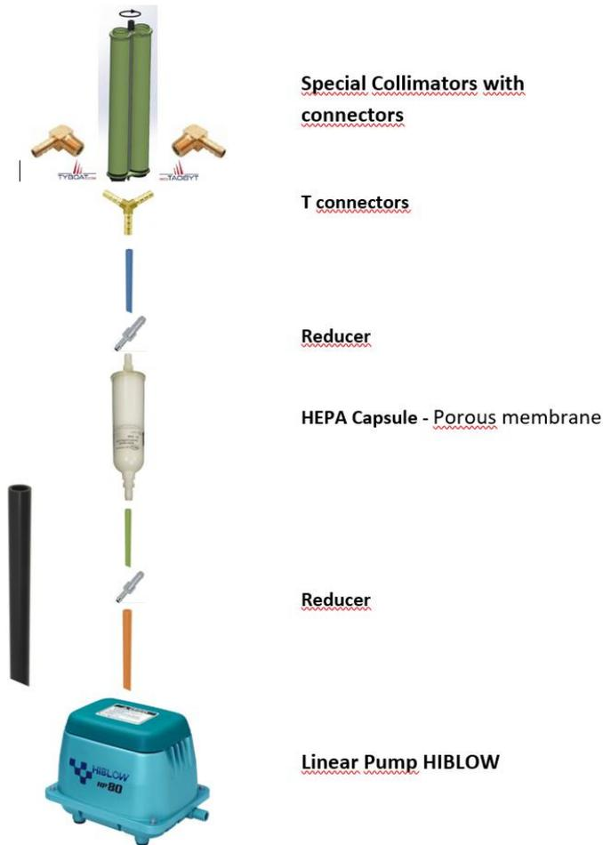
Figure 2 Schematic of the air pumping system
