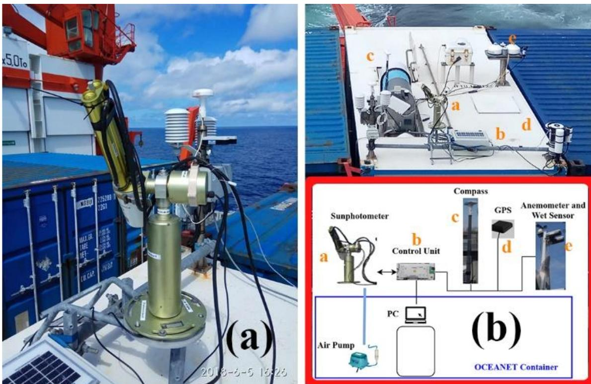
**Figure 1 picture of the optical head and tracking base over the OCEANET container and schematic.**
