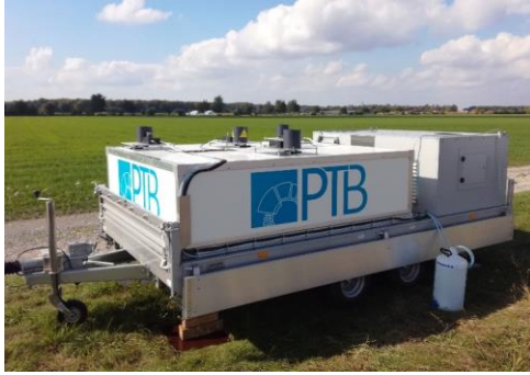
Figure 2: Photograph of the bistatic PTB lidar at the measurement site (opened trailer housing).
