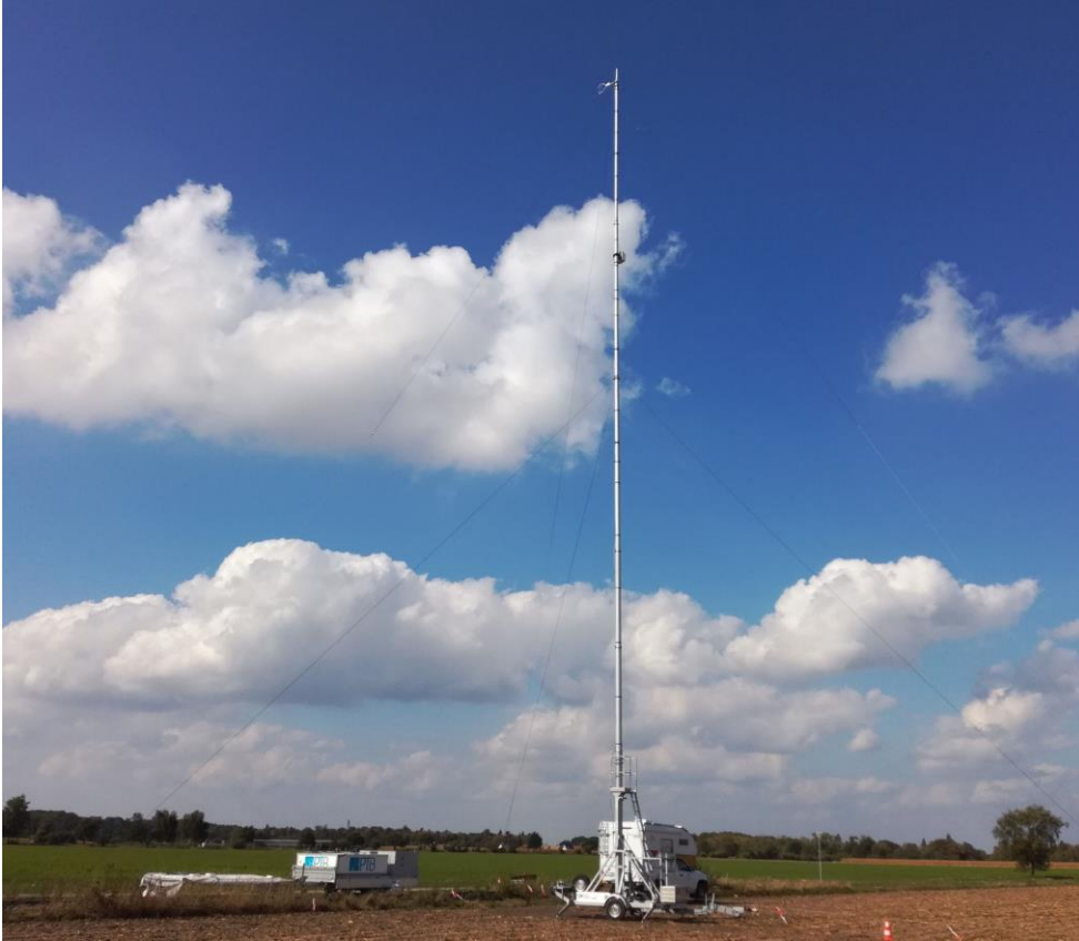
Figure 3: Photograph of the set-up of the field intercomparison experiment between the bistatic PTB lidar (left) and the CSAT3B mounted on a mobile 30 m telescopic mast (centre right). The camera is facing north-west.
