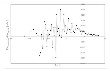
2. The H15 correction leads to an increase in cospectral energy density across all frequencies, but it does not effectively correct for this cospectral loss at high frequencies, which is the main reason for the discrepancies between the CSAT3B and the PTB lidar.
