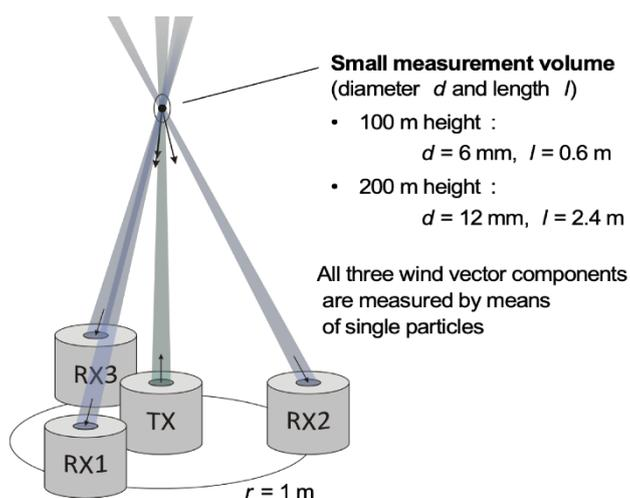
5 **Figure 1: Principle of the novel bistatic lidar consisting of one transmitting unit TX (green beam) and three receiving units RX**
