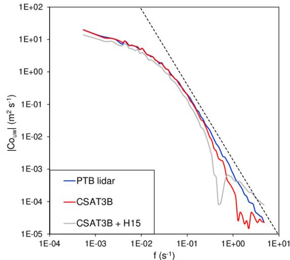
5 **Figure 8: Ensemble cospectra between  $u$  and  $w$  (absolute value) based on turbulence measurements from the PTB lidar and the CSAT3B sonic anemometer. The dashed line indicates the theoretical  $-7/3$  power law in the inertial subrange.**
