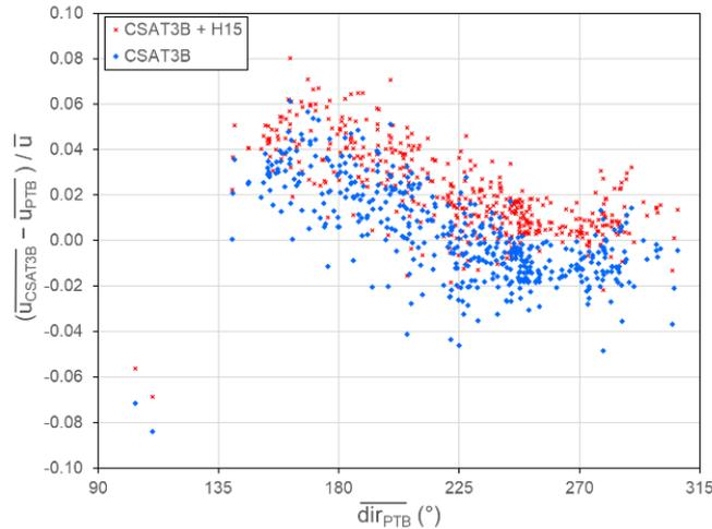
**Figure 6: Differences in wind velocity measurements between the two instruments  $\bar{u}$ , normalized by the mean wind velocity in  $\Delta\bar{u}/\bar{u}$  versus the wind direction  $dir$ . The CSAT3 data are shown with and without the H15 correction.**
