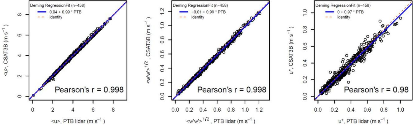
**Figure 5:** Comparison for mean wind velocity (left), standard deviation of the vertical velocity component (centre), and friction velocity (right), including the regression equation and correlation coefficient. A solid blue line indicates the Deming regression and the dashed red line indicates identity.
