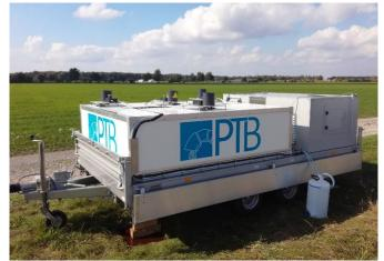
Figure 2: Photograph of the bistatic PTB lidar at the measurement site (opened trailer housing).
