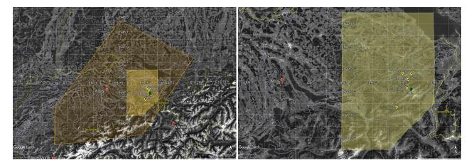
**Figure 1.** Left: Approximate extent of the maximum area covered by the LMA (Orange poligon). The yellow area shows the region with more comprehensive coverage. Radar positions are marked by red dots while the position of the LMA sensors is marked by yellow dots. The Säntis tower is marked by a green dot. Right: Zoom over the best covered area
