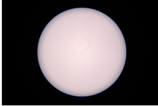
Figure 3: We captured a reference image inside the uniformly-illuminated integrating sphere.
