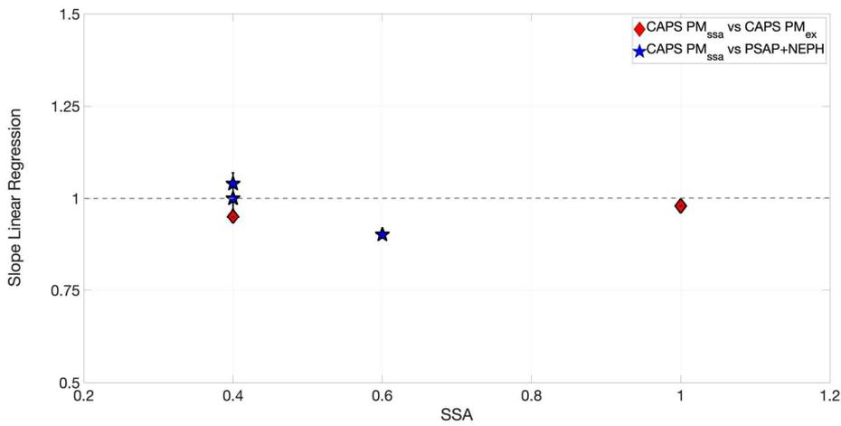
285 **Figure 7. Slope values of the linear regressions of measured particle extinction as a function of nominal aerosol SSA for the different instrument intercomparison.**
