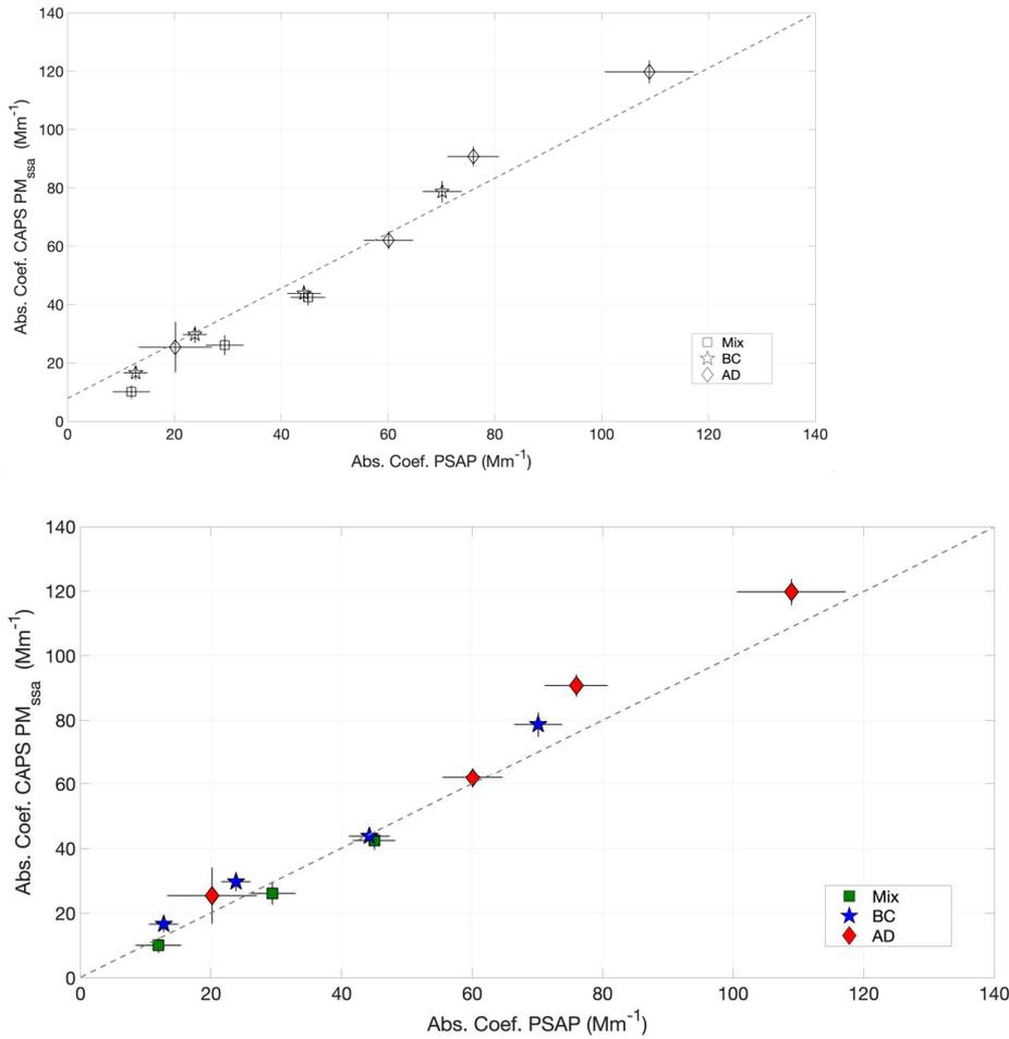
Figure 13. Comparison result of the absorption indirect measurement by the CAPS PM<sub>ssa</sub> with the measurements from the PSAP for AD, BC and Mixture, (dashed line is the identity line (i.e., 1:1 line)).
