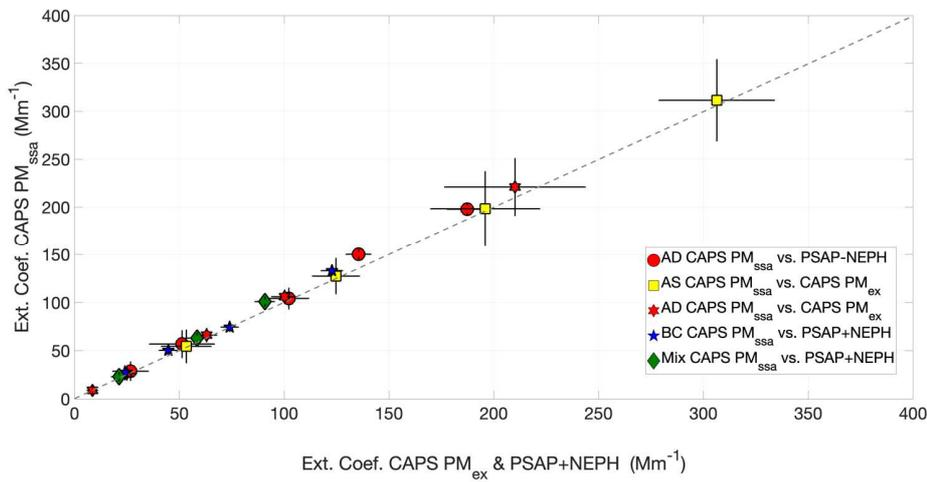
Figure 6. Comparison result of the extinction channel of the CAPS PM<sub>ssa</sub> with the CAPS PM<sub>ex</sub> and the combination PSAP+NEPH for for the different aerosol types (dashed line is the identity line (i.e., 1:1 line)).
