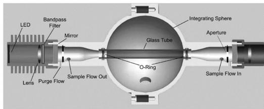
**Figure 3. CAPS PM<sub>ssa</sub> components and set-up (Onasch et al., 2015).**
