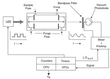
**Figure 2. Overview of the main components and operation principle of the CAPS PM<sub>ex</sub> instrument (Massoli et al., 2010)**
