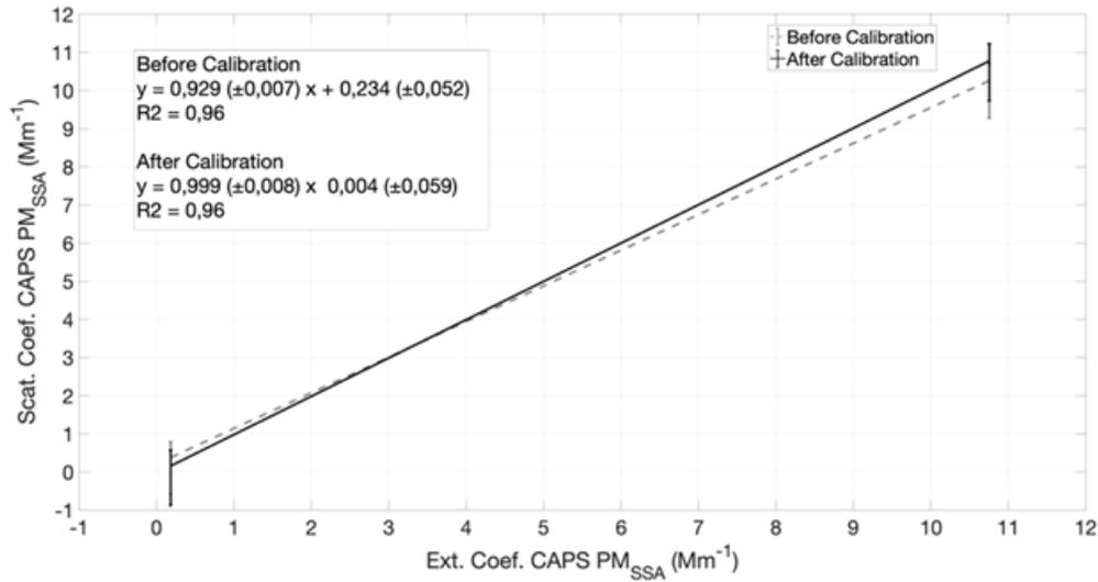
Figure 4. Scatterplot of the correlation of the extinction and scattering channel of the CAPS PMssa before and after the calibration using CO<sub>2</sub>.
