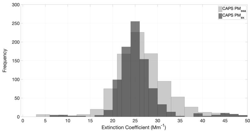
**Figure 8. Frequency of extinction coefficient measurement for the CAPS PM<sub>ssa</sub> and PM<sub>ex</sub> systems at the nominal 25 Mm<sup>-1</sup> (level 5) test point for AD.**
