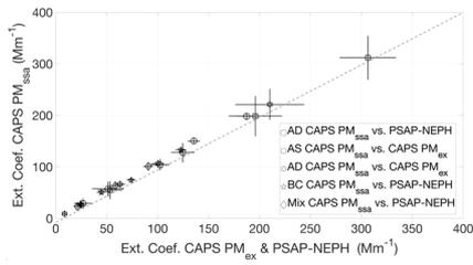
Figure 4. Comparison result of the extinction channel of the CAPS PM<sub>ssa</sub> with the CAPS PM<sub>ex</sub> and the PSAP-NEPH for for the different aerosol types.
