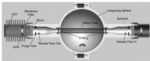
**Figure 2. CAPS PM<sub>SSA</sub> components and set-up (Onasch et al., 2015).**
