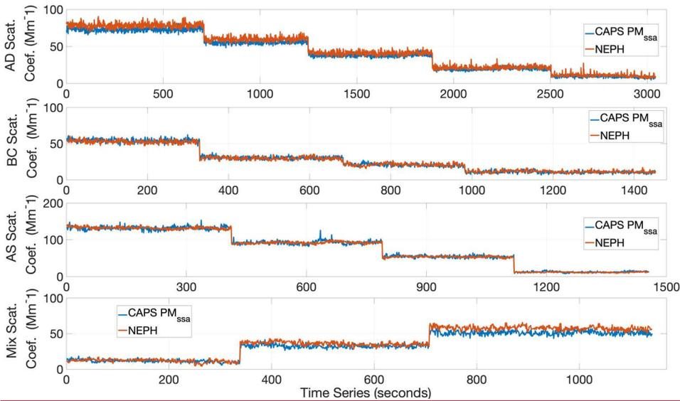
**Figure 9. Time series of the measurements by the scattering channel coefficients parallel measured by the different instruments: CAPS PM<sub>ssa</sub> and NEPH for the different aerosol types (BC (top-) AS(middle-) and Mix (bottom-figure)).**
