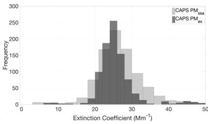
Figure 6. Frequency of extinction coefficient measurement for the CAPS PM<sub>ssa</sub> and PM<sub>ex</sub> systems at the nominal 25 Mm<sup>-1</sup> (level 5) test point for AD.
