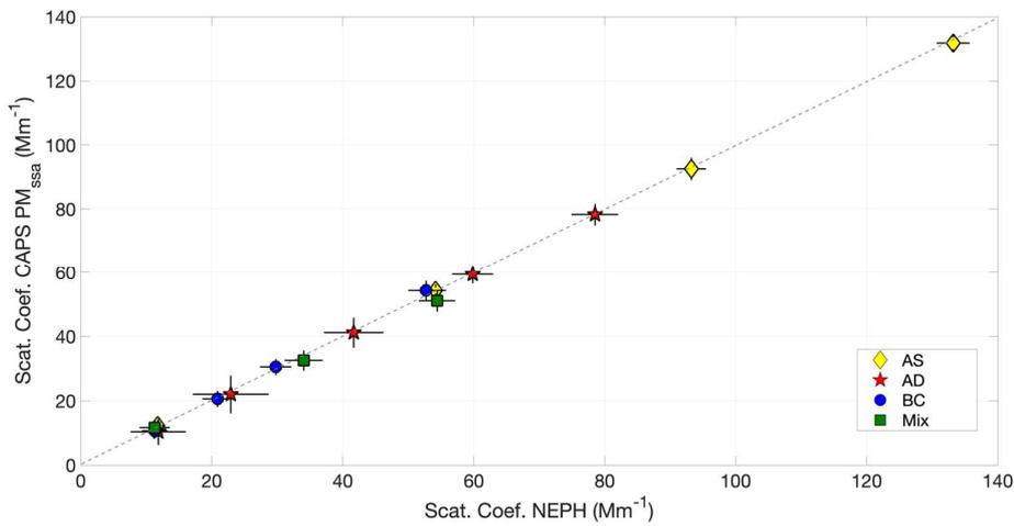
Figure 10. Comparison result of the scattering channel of the CAPS  $PM_{ssa}$  with the measurements from the NEPH for the different aerosol types (dashed line is the identity line (i.e., 1:1 line)).
