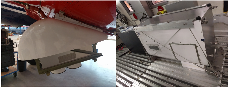
Figure 3. Left: MiRAC-A with opened belly pod below the research aircraft Polar 5. Right: MiRAC-P eight channel radiometer mounted in the aircraft cabin.
