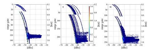
Figure 1. Sensitivity limit in [dBz] ( $Z_{min}$ ) for vertical polarization of different chirp tables with different vertical resolution as a function of distance from the aircraft (secondary y-axes) for the three settings used during ACLOUD. The vertical resolution increases from a) to c) with increasing number of range gates, a) 154 range gates, May 25, 08:58 - 12:19 UTC, RF05, b) 242 range gates June 23, 12:53 - 13:43 UTC, RF22, c) 364 range gate May 27, 08:14 - 11:04 UTC, RF06.
