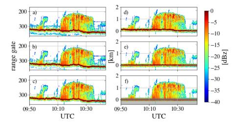
Figure 5. Time series of  $Z_e$  profiles measured during RF06 on May 27 2017 for different processing steps (see Table 3): a) raw data, b) after subtraction of mirror signal, c) after speckle filter, d) filtered data on a time-height grid, e) corrected for sensor altitude, mounting position, pitch and roll angle, f) remapping onto a constant vertical grid. The grey shading indicates the range of surface contamination ( $\leq 150 \text{ m}$ ).
