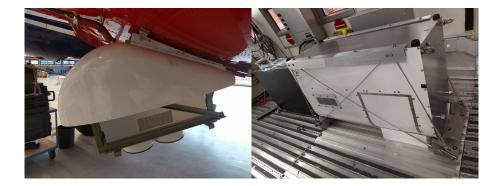
**Figure 3.** Left: MiRAC-A with opened belly pod below the research aircraft Polar 5. Right: MiRAC-P eight channel radiometer mounted in the aircraft cabin.
