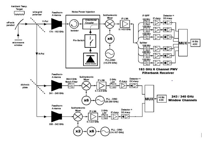
Figure 2. Block diagram of MiRAC-P.
