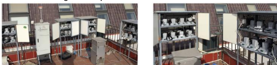
Figure (not included in manuscript): Co-location of 60 PAMs at PKU during the heating and non-heating season for a four-week period. PAMs were placed in custom-made protective shelters in proximity to the inlets of reference instruments and were connected on mains.
