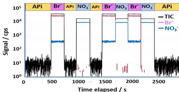
**Figure 2** Demonstrating switching between multiple ion chemistries. Abbreviations used: *APi* = ambient ion mode, *Br* = bromide ion mode, *NO<sub>3</sub>* = nitrate ion mode, *TIC* = total ion count.
