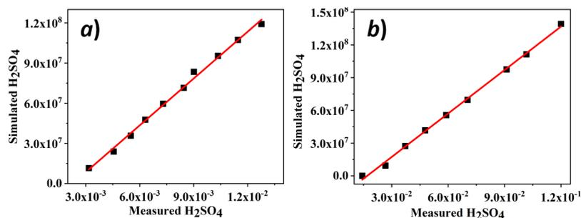
200 **Figure 3** Sulfuric acid (H<sub>2</sub>SO<sub>4</sub>, SA) calibration plots showing the simulated values against the measured ion signals
