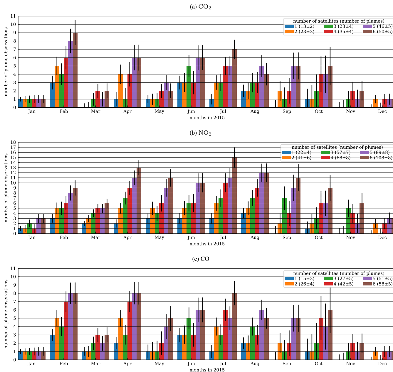
Figure 6. Number of cloud-free plumes of the city of Berlin with at least 100 pixels per month for (a) CO 2 , (b) NO 2 and (c) CO. The cloud threshold is 1% for CO 2 , 30% for NO 2 and 5% for CO observations. Error bars are obtained by comparing all available satellites. The number of expected plumes per satellite is 8, 17 and 9 for the CO 2 , NO 2 and CO instrument, respectively.
