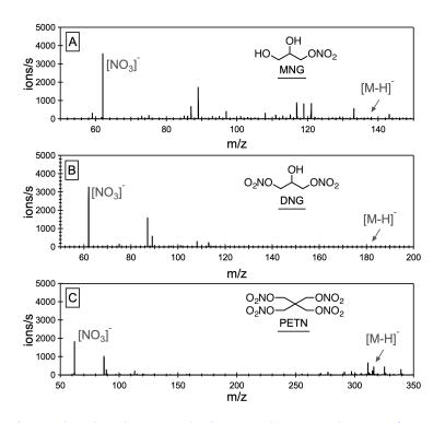
The figure above shows that the nitrate explosives produce mostly NO<sub>3</sub><sup>-</sup> fragments but very little molecular ions on their own if directly infused into negative electrospray.
