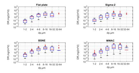
**Figure 6**: Box-plots of size resolved deposition rate (campaign data; Flat plate, Sigma-2, MWAC and BSNE samplers). On each blue box, the central mark is the median, the edges of the box are the 25th and 75th percentiles. The red vertical lines show the standard deviation. The median, percentiles and standard deviations shown there correspond to the variability of the whole campaign for each
