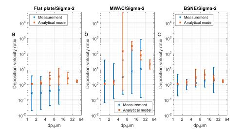
**Figure 8**: Comparison of geometric mean ratio of deposition velocities for different sampler pairs derived from measured deposition rates (blue) and from corresponding deposition models (orange).
