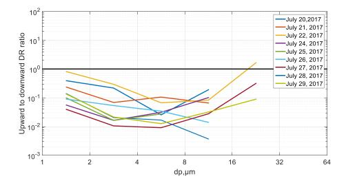
**Figure 14**: Ratio of upward- to downward-directed mass deposition rate as function of particle size. The deposition rate is measured using the upward-downward-Flat plate sampler (with 25 mm stub).
