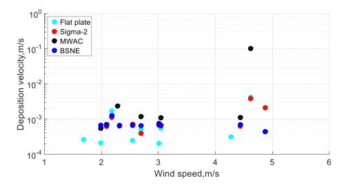
**Figure 9**: Apparent deposition velocity: ratio of number deposition rate determined from SEM measurements to the number concentration observed by the OPC as function of wind speed. For the consideration, only the overlapping size range (approximately 1-10 μm) was used.
