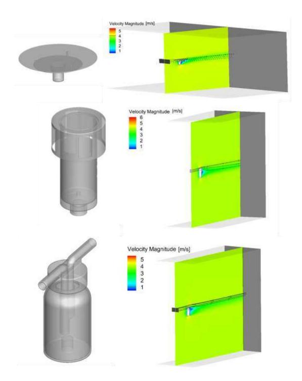
**Figure 3**: Geometries of Flat plate sampler (top), Sigma-2 sampler (middle), MWAC sampler (bottom). CFD modeling domain and velocity magnitude, inlet velocity: 4 m/s (right); in addition, the injection area is shown in black (Flat plate sampler: width 0.2 m, height 0.05 m; Sigma-2-sampler: width 0.2 m, height 0.1 m; Bottle sampler: width 0.1 m, height 0.05 m) along with exemplary streamtraces.
