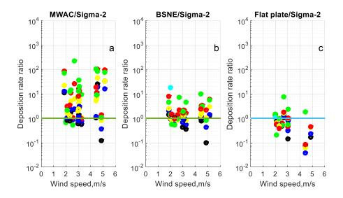
**Figure 7**: Deposition rate ratio as function of wind speed for different days (MWAC/ Sigma-2 (a), BSNE/Sigma-2 (b) and BSNE/ Sigma-2 (c)). Different colors represent deposition rate measured in different size intervals (black: 1-2 μm; blue: 2-4 μm; yellow: 4-8 μm; red: 8-16 μm; green: 16-32 μm; cyan: 32-64 μm).
