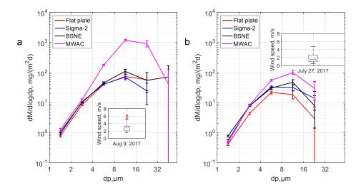
**Figure 5**: Size resolved mass deposition rate measured by different passive samplers: a) dust event day; b) non-dust event day. Data are derived from SEM measurements. **The bars show the central 95% confidence interval of the daily variation.** The inserts show box plots for the wind speed distribution based on 30-min intervals.
