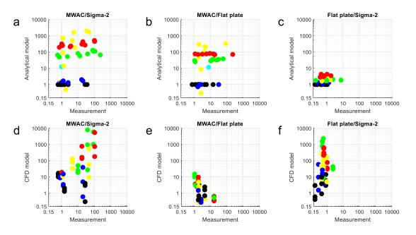
**Figure 16**: Comparison of the observed deposition velocity ratios with modeled ones by the analytical deposition models (upper row, a-c) and by the CFD models (lower row, d-f). (a, d) MWAC/Sigma-2; (b, e) MWAC/Flat plate; (c, f) Flat plate/Sigma-2. Multiple daily measurements are shown in each plot. Different colors represent different size intervals. 1-2 μm: Black, 2-4 μm: Blue, 4-8 μm: Yellow, 8-16 μm: Red, 16-32 μm: Green, 32-64 μm: Cyan.
