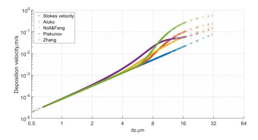
**Figure 2**: Deposition velocities for single particles to a smooth surface (Flat plate sampler) calculated by using set of different classical deposition models for Tenerife samples (Aug 9, 2017; average wind speed =3.0 m/s).
