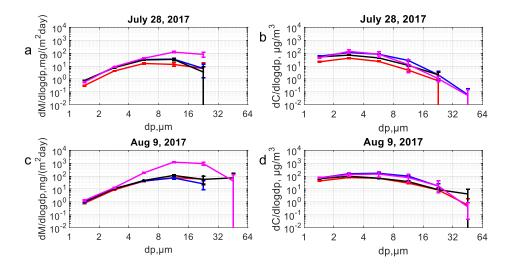
**Figure 10**: Comparing different samplers with respect to (a, c) dust mass deposition rates and (b, d) dust mass concentrations calculated from application of the corresponding model as function of particle size. Different colors indicate different samplers (red: Flat plate; blue: Sigma-2; black: BSNE and magenta: MWAC). The bars show the central 95% confidence interval of the daily variation. According deposition models for concentration calculation are given in the **Table 1**.
