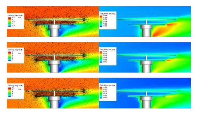
**Figure 4**: Flat plate Sampler: Velocity magnitude and turbulence intensity at wind speed 2 m/s (top), Flat plate Sampler: Velocity magnitude and turbulence intensity at wind speed 4 m/s (middle), Flat plate Sampler: Velocity magnitude and turbulence intensity at wind speed 8 m/s (bottom).
