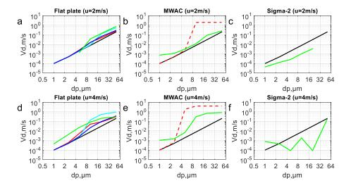
**Figure 15**: Deposition velocities calculated for different samplers by analytical and CFD approaches. The red curve shows the deposition velocity calculated using the Piskunov model, the dotted red curve shows the combination of the Piskunov and the impaction curve model, the black curve shows the Stokes deposition velocity, the blue curve the Noll and Fang model, the cyan the Zhang model, and the
