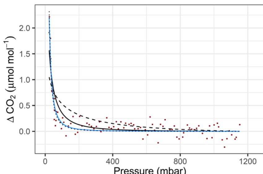
**Figure 2:** Measured and modelled amount fractions of  $\text{CO}_2$  for the aluminum cylinder from the QCLAS setup. Red points show measured data, black dashed lines show the modelled fit with  $K=0.001 \text{ bar}^{-1}$ , black lines show the modelled fit with  $K=0.01 \text{ bar}^{-1}$ , blue lines show the modelled fit with  $K=0.152 \text{ bar}^{-1}$  and black dotted lines show the modelled fit with  $K=1 \text{ bar}^{-1}$
