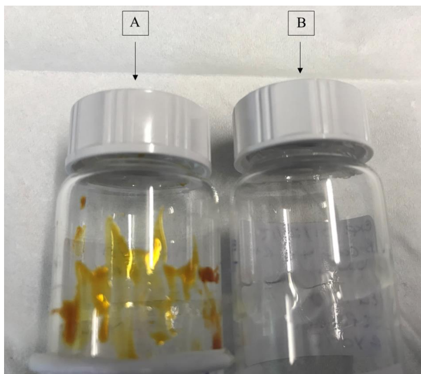
Figure 3 – Visual differences observed in the light absorbing properties of toluene (A) and \beta -caryophyllene SOA (B) formed under replicate experimental conditions (55% relative humidity with a VOC/NO x ratio of 13, exp. 36 and 31 (see Table 1), 5 respectively).
