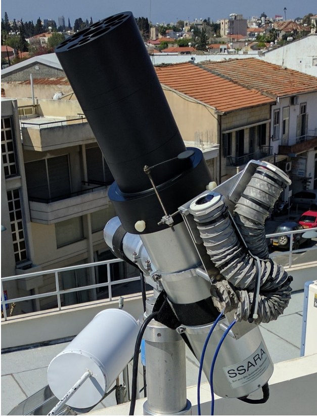
Figure 2. SSARA sensorhead on the alt-azimuthal mount with straylight baffle installed.
