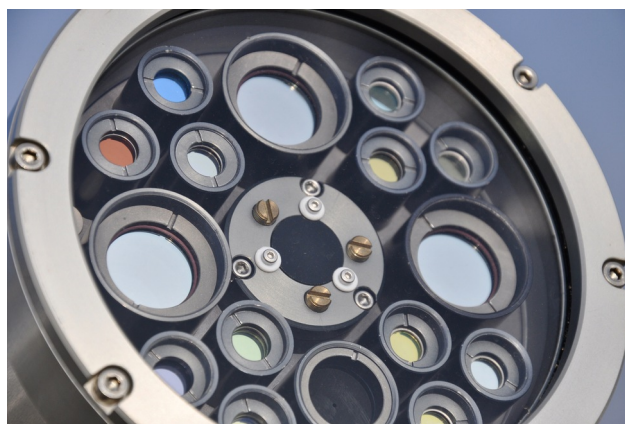
Figure 1. SSARA sensorhead with 12 direct channels (smaller diameter tubes), and 3 polarized channels (larger diameter at the top, left and right). The quadrant sun-tracker is in the center, below it is a finder for manual sun tracking.
