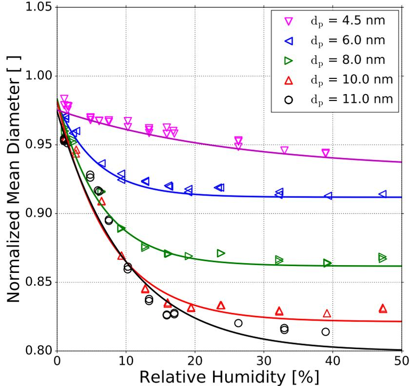
**Figure 4.** Normalized mean diameter of sodium chloride particles as a function of relative humidity which represents the shrinkage of NaCl seeds in the presence of water vapor. All sizes are mobility equivalent diameters. Each line represents a tentative three-parameter fit of an exponential decay. The measurements were conducted with SHT75 sensors with an accuracy of  $\pm 1.8\%$  RH and with a HMP35E probe with an accuracy of  $\pm 2.0\%$  RH.
