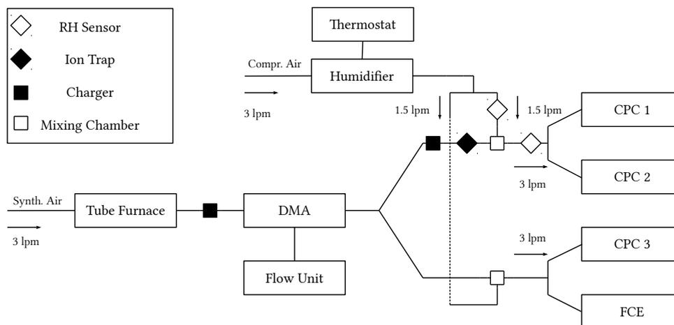
**Figure 1.** The experimental setup for evaluating the relative humidity dependent counting efficiency of continuous flow type CPCs (TSI 3776 UCPC), which was measured relative to a Faraday Cup Electrometer (FCE) (Wlasits, 2019).
