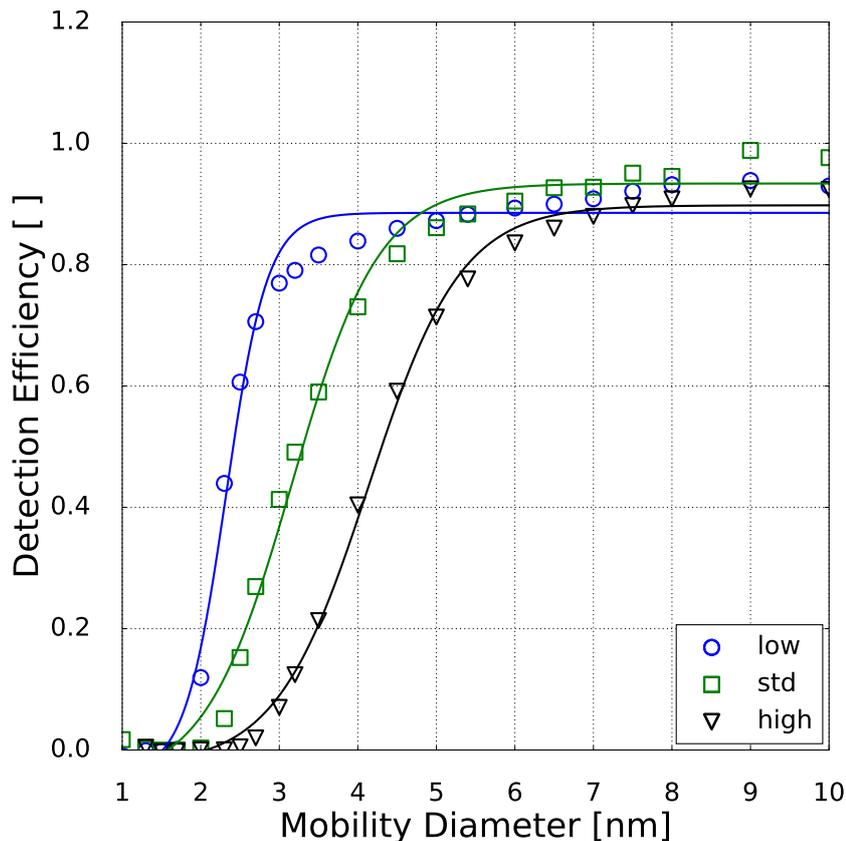
**Figure 5.** Detection efficiency as a function of mobility diameter for neutral sodium chloride particles. The symbols represent the measured counting efficiencies for low (circles), standard (std, squares) and high temperature (triangles) settings at 10% RH at room temperature of the inlet line. The line displays a fit to the measured counting efficiencies (Wiedensohler et al., 1997). Thereby the corresponding cut-off diameter with the detection efficiency of 0.5 can be evaluated.
