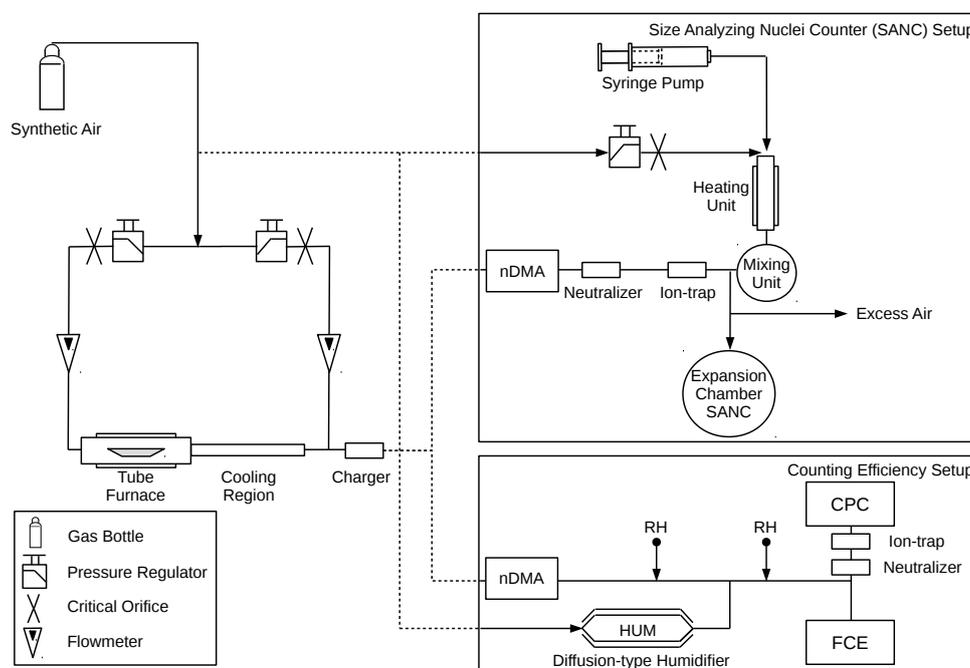
**Figure 1.** The experimental setup for evaluating the supersaturation and nucleation temperature with the SANC and the relative humidity dependent counting efficiency measurements of a continuous flow type CPC (TSI 3776 UCPC), which was measured by operating a Faraday Cup Electrometer (FCE) in parallel.
