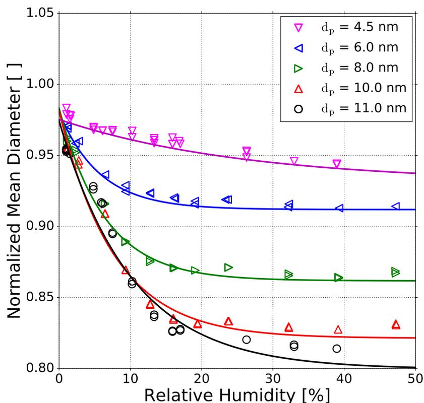
**Figure 4.** Normalized mean diameter of sodium chloride particles as a function of relative humidity which represents the shrinkage of NaCl seeds in the presence of water vapor. All sizes are mobility equivalent diameters. Each line represents a tentative three-parameter fit of an exponential decay.
