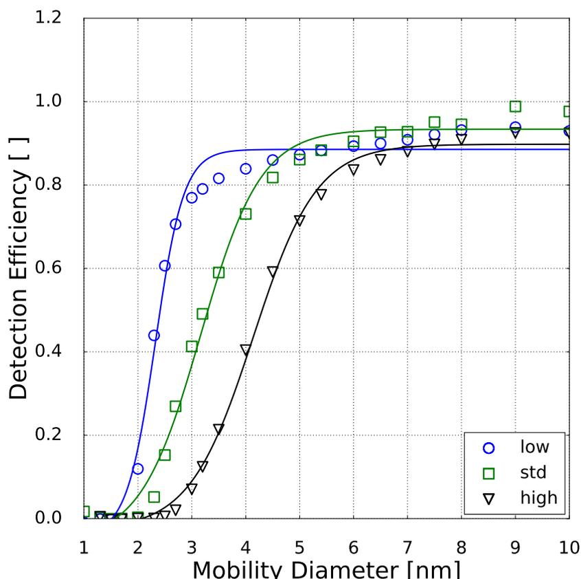
**Figure 5.** Detection efficiency as a function of mobility diameter for neutral sodium chloride particles. The symbols represent the measured counting efficiencies for low (circles), standard (std, squares) and high temperature (triangles) settings at 10% RH. The line displays a fit to the measured counting efficiencies (Wiedensohler et al., 1997). Thereby the corresponding cut-off diameter with the detection efficiency of 0.5 can be evaluated.
