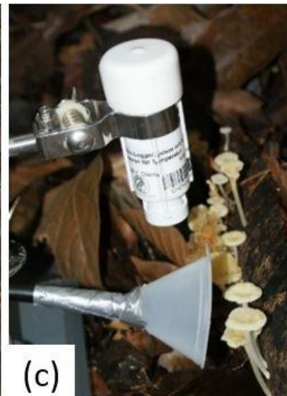
Figure 3: Setup used for field measurements. The optical particle sensor (OPS) is located in a box for weather protection. From this, an inlet ending with a funnel leads to the organism of interest. The setup is accompanied by a T/RH-sensor located in the direct vicinity of the sample (a) Schematic drawing, (b) overview photograph, and (c) close-up photograph of the described setup.
