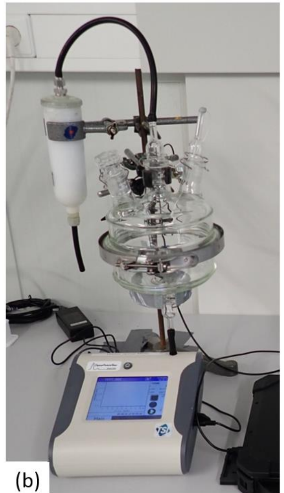
Figure 4: Setup used for laboratory experiments. The samples are placed in a glass cuvette in a vertical air stream. Air is supplied via an inlet with a filter connected to it; the outlet is connected to an OPS for particle measurements. A humidity and temperature sensor is placed inside the cuvette through an opening in the upper lid, which is sealed to avoid contamination. (a) Schematic drawing, and (b) close-up photograph.
