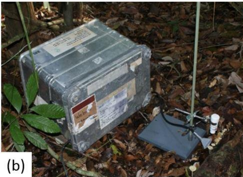
Figure 3: Setup used for field measurements. The optical particle sensor (OPS) is located in a box for weather protection. From this, an inlet ending with a funnel leads to the organism of interest. The setup is accompanied by a temperature and humidity (T/RH) sensor located in the direct vicinity of the sample (a) Schematic drawing, (b) overview photograph, and (c) close-up photograph of the described setup.
