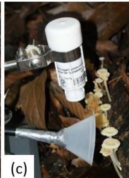
Figure 3: Setup used for field measurements. The optical particle sensor (OPS) is located in a box for weather protection. From this, an inlet ending with a funnel leads to the organism of interest. The setup is accompanied by a temperature and humidity (T/RH) sensor located in the direct vicinity of the sample (a) Schematic drawing, (b) overview photograph, and (c) close-up photograph of the described setup.
