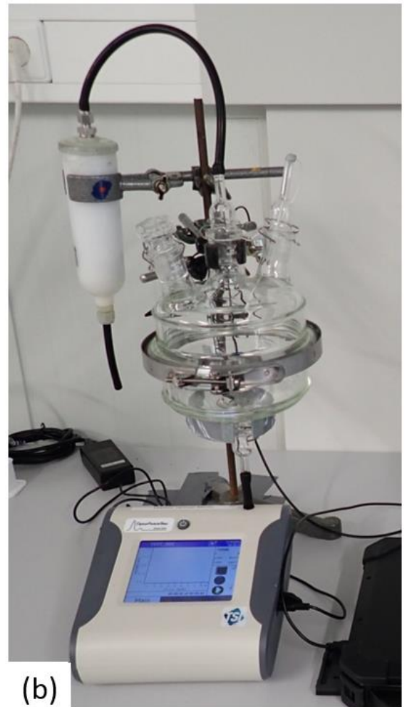
Figure 4: Setup used for laboratory experiments. The samples are placed in a glass cuvette in a vertical air stream. Air is supplied via an inlet with a filter connected to it; the outlet is connected to an OPS for particle measurements. A temperature and humidity (T/RH) sensor is placed inside the cuvette through an opening in the upper lid, which is sealed to avoid contamination. (a) Schematic drawing, and (b) close-up photograph.
