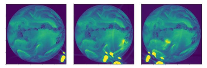
Figure 8. Three sequential images affected by the direct straylight anomaly.
