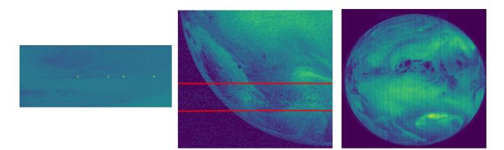
**Figure 3.** Examples of low quality sensory data. Left: a scanline contains an interference pattern. Center: a block of scanlines (inside the red lines) with a much lower signal-to-noise ratio than neighbouring scanlines. Right: image contains an unknown disturbance pattern.
