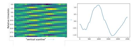
**Figure 10.** Example of the Meteosat 5 optical hardware issue in time, where the left image shows the anomaly's bias for consecutive images across the scanlines. The right image is for a particular timeslot and shows the anomaly's bias across the scanlines.
