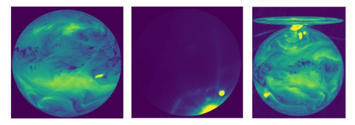
Figure 7. Three examples of the direct straylight effect anomaly.
