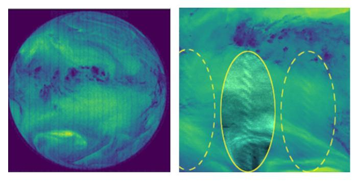
**Figure 5.** Two examples of the "suspicious pattern" anomaly: In the left image the vertical stripes are visible. In the right image the ovals indicate the position of the suspicious pattern; the middle oval has been altered to enhance visibility of the pattern.
