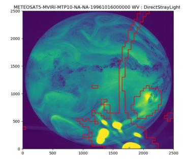
Figure 9. Segmentation result of the direct straylight anomaly detection.
