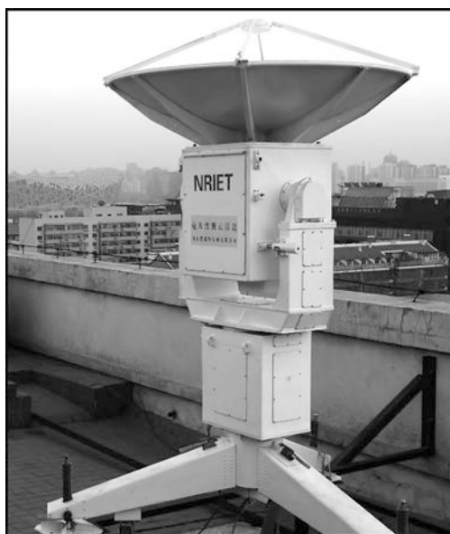
120 Fig. 1. The Ka-band polarization Doppler radar at the Institute of Atmospheric Physics, Chinese Academy of Physics, Beijing, China (39.967°N, 116.367°E).
