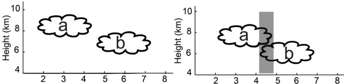
In the left figure, final radar CTH is the average CTH of all cloudy profiles of cloud 'a' and cloud 'b'. In the right figure, final radar CTH is the average CTH of all cloudy profiles of cloud 'a' and part cloudy profiles of cloud 'b' (where cloudy profiles in the gray frame are not included). We did not use the mean CTH of the upper-level cloud 'a' as final radar CTH because that might bring more bias to what satellite measures within an area.
