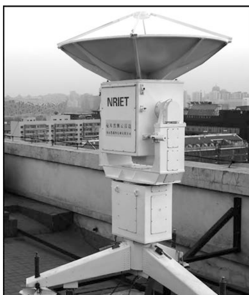
120 Fig. 1. The Ka-band polarization Doppler radar at the Institute of Atmospheric Physics, Chinese Academy of Sciences , Beijing, China (39.967°N, 116.367°E).
