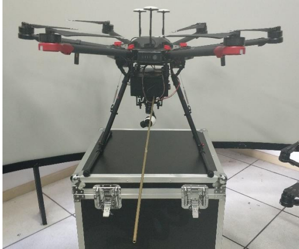
Figure 1. Image of the modified UAV platform. The black box installed under the UAV is a pod which was designed and customized by us. It carries a gas pump (to collect the ship's exhaust), gas circuit, a filter (to remove water vapor), sensors for SO 2 and CO 2 , a small motor (to provide energy for pumping), a camera, and communication modules.
