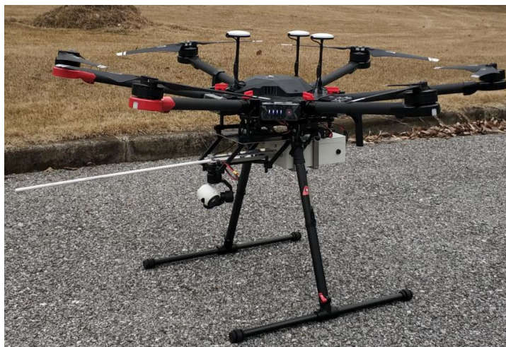
Figure 1 The second-generation pod (the volume gets smaller)
