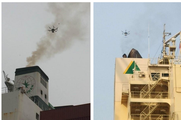
Figure 4. Photographs showing the flight of the UAV during measurements. The UAV platform was flown close to the funnel of ship for collecting exhaust gas and detection at Waigaoqiao pier.
