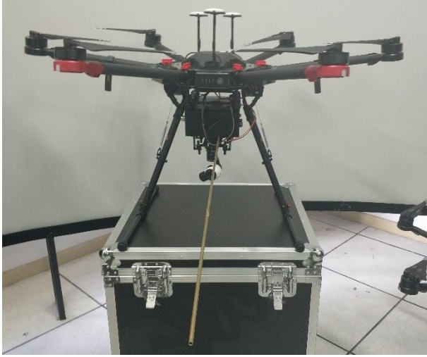
5 Figure 1. Image of the modified UAV platform. The black box installed under the UAV is a pod which was designed and customized by us. It carries a gas pump (to collect the ship's exhaust gas ), gas circuit, a filter (to remove water vapor), sensors for SO 2 and CO 2 , a small motor (to provide energy for pumping), a camera, and communication modules.
