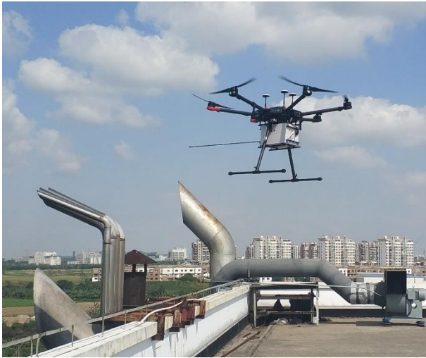
Figure 2. UAV platform flying close to the smoke stack for collecting exhaust gas in the automatic engine room laboratory of Shanghai Maritime University.
