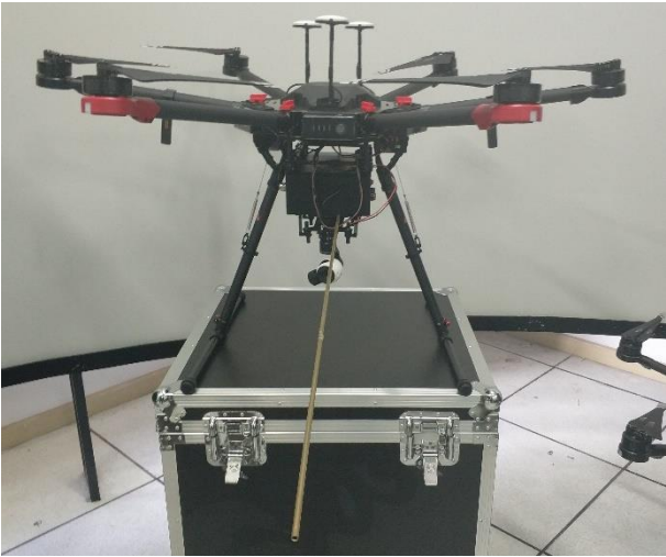
Figure 1. Image of the modified UAV platform. The black box installed under the UAV is a pod which was designed and customized by us. It carries a gas pump (to collect the ship's exhaust gas ), gas circuit, a filter (to remove water vapor), sensors for SO 2 and CO 2 , a small motor (to provide energy for pumping), a camera, and communication modules.
