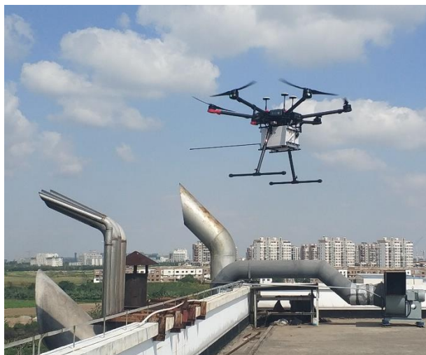
10 Figure 2. UAV platform flying close to the smoke stack for collecting exhaust gas in the automatic engine room laboratory of Shanghai Maritime University.
