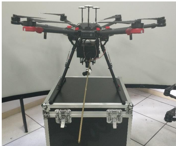
Figure 1. Image of the modified UAV platform. The black box installed under the UAV is a pod which was designed and customized by us. It carries a gas pump (to collect the ship's exhaust), gas circuit, a filter (to remove water vapor), sensors for \text{SO}_2 and \text{CO}_2 , a small motor (to provide energy for pumping), a camera, and communication modules.
