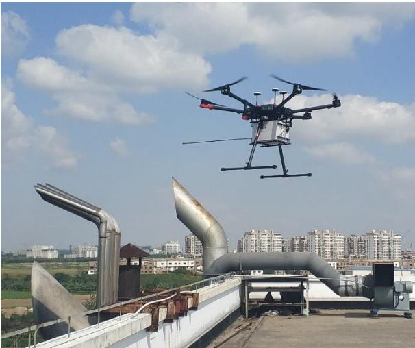
Figure 2. UAV platform flying close to the smoke stack for collecting exhaust gas in the automatic engine room laboratory of Shanghai Maritime University.
