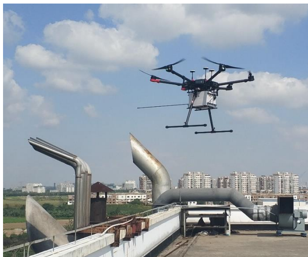
5 Figure 2. UAV platform flying close to the smoke stack for collecting exhaust gas in the automatic engine room laboratory of Shanghai Maritime University.
