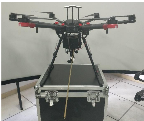
Figure 1. Image of the modified UAV platform. The black box installed under the UAV is a pod which was designed and customized by us. It carries a gas pump (to collect the ship's exhaust gas), gas circuit, a filter (to remove water vapor), sensors for \text{SO}_2 and \text{CO}_2 , a small motor (to provide energy for pumping), a camera, and communication modules.
