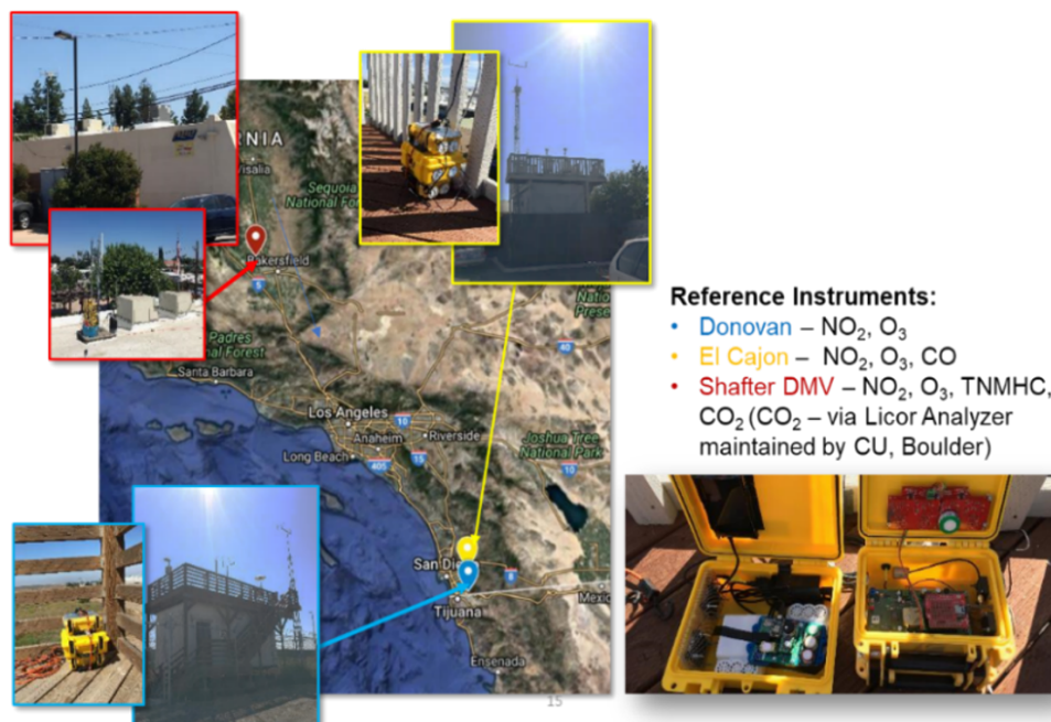
Figure 1. Map and images of deployment locations. Shafter DMV (red) was located 250 mi away from Donovan (blue) and El Cajon (yellow), which were located in San Diego, CA. (bottom right) Deployment containers configuration for the extended deployment. Each container has active ventilation to keep the internal conditions equivalent to the ambient environment.
