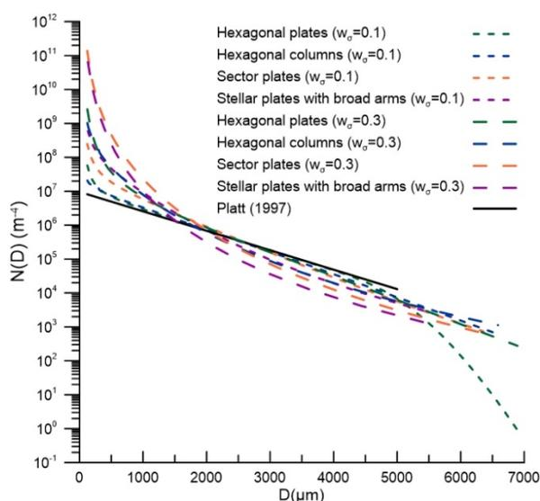
Figure 5. PSDs retrieved from Doppler spectra affected by turbulence shown in fig. 4b. The solid black line is the PSD given by Platt (1997) at  $-10^{\circ}\text{C}\sim-5^{\circ}\text{C}$  (same as fig. 4a).
