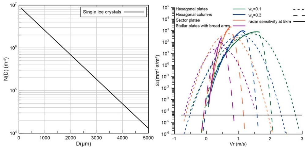
Figure 4. (a) Exponential distribution used in this paper. (b) The Doppler spectral density calculated from the exponential distribution without turbulence (the solid line) and at different turbulence intensities (the dashed line). Radar sensitivity at 5 km of M3 are marked by a solid black line.
