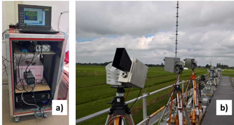
Figure 1. The IMPACT instrument installed during CINDI-2. a) Indoor parts integrated into a 19" rack. b) Telescope unit on top of the container deck (foreground). Next to IMPACT is the IUP-Bremen 2D-MAX-DOAS instrument (background) used for comparison in Sect. 4.1.
