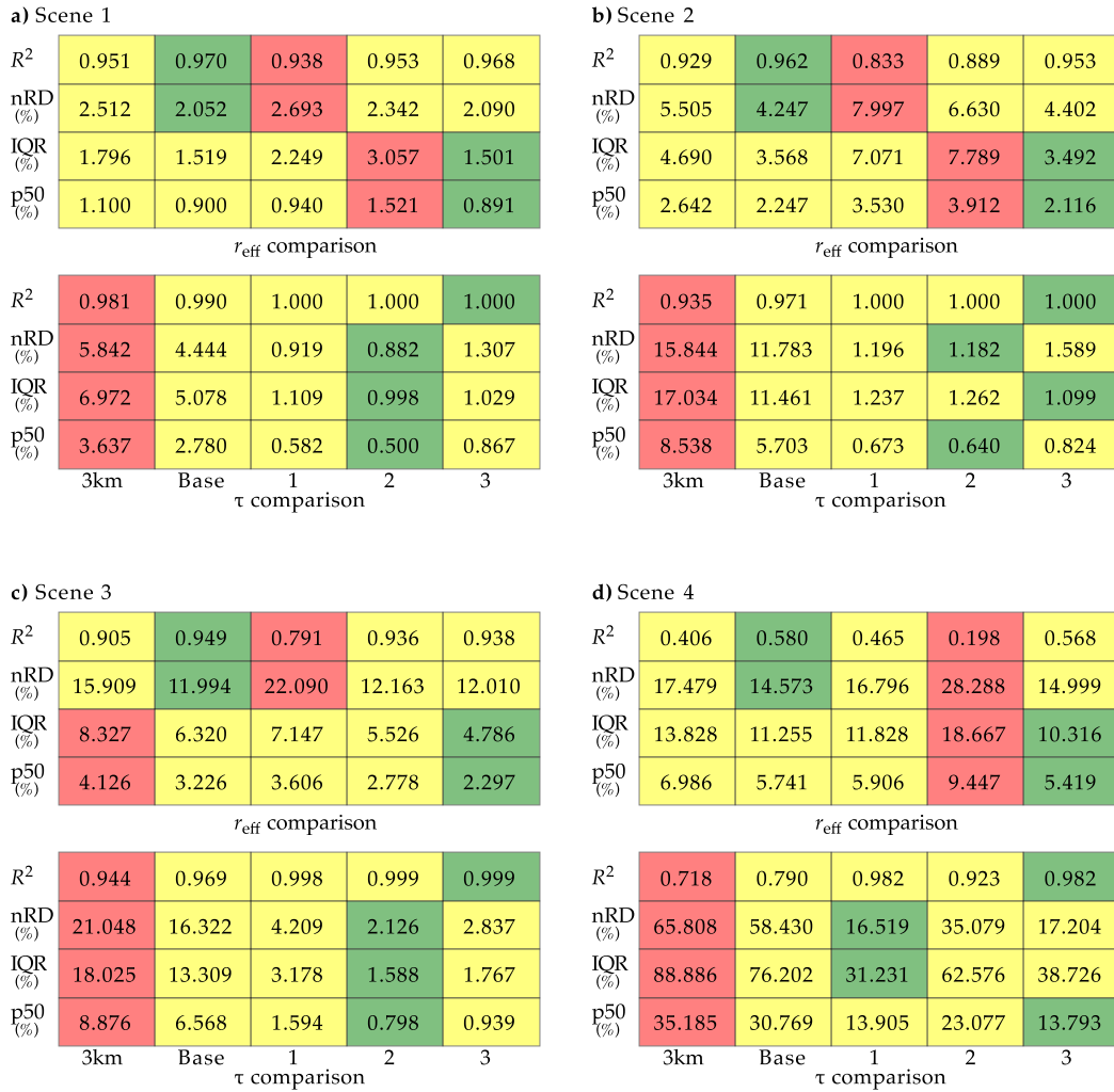
Figure 8. (a) Comparison of retrieved cloud optical thickness ( \tau , bottom panels) and effective droplet radius ( r_{\text{eff}} , top panels) from the native 3 LRES resolution (at a scale of \approx 3 km resolution ) and baseline retrievals (i.e., only accounting for low-resolution reflectance variability), as well as the various downscaling experiments 1 ( 1b statistical downscaling approach), 2b 2 (Constant Reflectance Ratio Approach), 3b , 3c , and 3d 3 (Adjusted Lookup Table Approach with LUT Slope Adjustment), and the reference retrieval results. Parameters to quantify the comparisons are the median of the relative difference to the reference (p50), relative interquartile range (IQR; 75 th -25 th percentile of the relative difference to the reference), normalized root-mean-square deviation (nRD; defined as the RD between the two data sets, normalized by the average reference retrieval), and the explained variance ( R^2 ). Green colors indicate the experiment that compares best to the reference results, i.e., highest R^2 and lowest p50, IQR, and nRD. Red colors indicate the experiment with the worst agreement to the reference retrievals, while yellow colors indicate all experiments in between. Data is from example scene 1 sampled on 1 June 2013 sampled at 10:05 UTC. (b)–(d) Same as (a) but for example scene 2 to 4, respectively.
