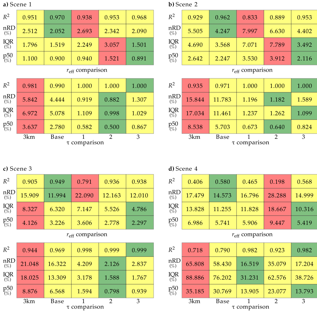
Figure 8. (a) Comparison of retrieved cloud optical thickness ( \tau , bottom panels) and effective droplet radius ( r_{\text{eff}} , top panels) from the native LRES resolution (at a scale of \approx 3 km) and baseline retrievals (i.e., only accounting for low-resolution reflectance variability), as well as the downscaling experiments 1 (statistical downscaling approach), 2 ( Constant Reflectance Ratio Approach ), and 3 ( Adjusted Lookup Table Approach with LUT Slope Adjustment ), and the reference retrieval results. Parameters to quantify the comparisons are the median of the relative difference to the reference (p50), relative interquartile range (IQR; 75 th -25 th percentile of the relative difference to the reference), normalized root-mean-square deviation (nRD; defined as the RD between the two data sets, normalized by the average reference retrieval), and the explained variance ( R^2 ). Green colors indicate the experiment that compares best to the reference results, i.e., highest R^2 and lowest p50, IQR, and nRD. Red colors indicate the experiment with the worst agreement to the reference retrievals, while yellow colors indicate all experiments in between. Data is from example scene 1 sampled on 1 June 2013 sampled at 10:05 UTC. (b)–(d) Same as (a) but for example scene 2 to 4, respectively.
