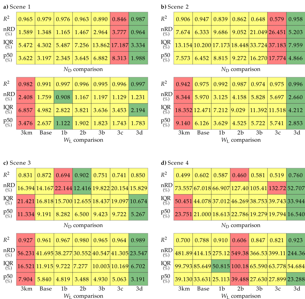
Figure 12. (a) Comparison of derived liquid water path ( W_L , bottom panels) and droplet number concentration ( N_D , top panels) from the native 3 km resolution and baseline retrievals, as well as the various downscaling experiments (1b, 2b, 3b, 3c, and 3d), and the respective reference results. Parameters to quantify the comparisons are the median of the relative difference to the reference (p50), relative interquartile range (IQR; 75 th -25 th percentile of the relative difference to the reference), normalized root-mean-square deviation (nRD; defined as the RD between the two data sets, normalized by the average reference retrieval), and the explained variance ( R^2 ). Green colors indicate the experiment that compares best to the reference results, i.e., highest R^2 and lowest p50, IQR, and nRD. Red colors indicate the experiment with the worst agreement to the reference retrievals, while yellow colors indicate all experiments in between. Data is from example scene 1 sampled on 1 June 2013 sampled at 10:05 UTC. (b)–(d) Same as (a) but for example scenes 2 to 4, respectively.
