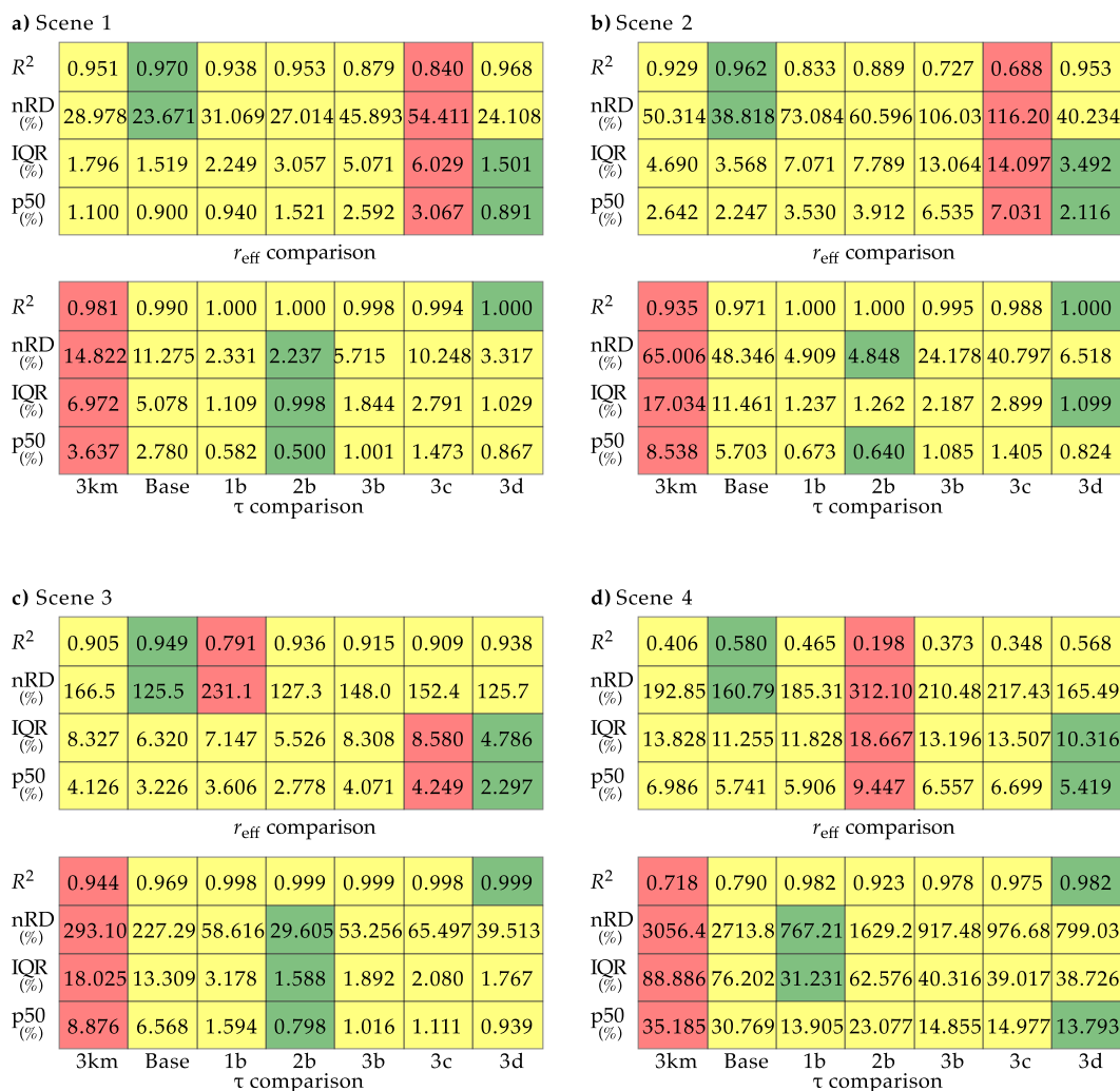
Figure 10. (a) Comparison of retrieved cloud optical thickness ( \tau , bottom panels) and effective droplet radius ( r_{\text{eff}} , top panels) from the native 3 km resolution and baseline retrievals (i.e., only accounting for low-resolution reflectance variability), as well as the various downscaling experiments (1b, 2b, 3b, 3c, and 3d), and the reference retrieval results. Parameters to quantify the comparisons are the median of the relative difference to the reference (p50), relative interquartile range (IQR; 75 th -25 th percentile of the relative difference to the reference), normalized root-mean-square deviation (nRD; defined as the RD between the two data sets, normalized by the average reference retrieval), and the explained variance ( R^2 ). Green colors indicate the experiment that compares best to the reference results, i.e., highest R^2 and lowest p50, IQR, and nRD. Red colors indicate the experiment with the worst agreement to the reference retrievals, while yellow colors indicate all experiments in between. Data is from example scene 1 sampled on 1 June 2013 sampled at 10:05 UTC. (b)–(d) Same as (a) but for example scene 2 to 4, respectively.
