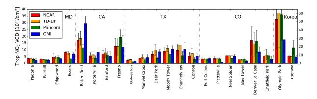
Figure 9. Site mean tropospheric  $NO_2$  VCDs calculated from NCAR (blue), TD-LIF (orange), Pandora (green), and OMI (blue) instruments. The OMI data are derived using observed  $NO_2$  profiles and downscaled using high-resolution model simulations. The vertical bars represent the standard deviations. A different y scale (on right,  $0-65 \times 10^{15}$  molec./cm<sup>2</sup>) is used for Korea.
