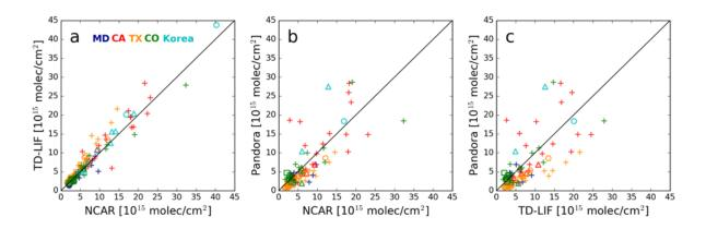
**Figure 6.** Comparison of NO<sub>2</sub> tropospheric columns derived from NCAR, TD-LIF, and Pandora instruments. Different colors represent the campaign location, and the symbols represent the type of surface monitors (open circle: photolytic converter, plus: molybdenum converter, triangle: CAPS, and square: CRDS).
