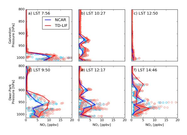
**Figure 7.** Vertical distribution of NO<sub>2</sub> mixing ratios at different local solar time (LST) over Galveston (top) and Deer-Park (bottom) in TX measured by the NCAR (light blue) and TD-LIF (orange) instruments. The circles in lighter colors represent 1-second measurements, and the solid lines show the mean values for NCAR (blue) and TD-LIF (red).
