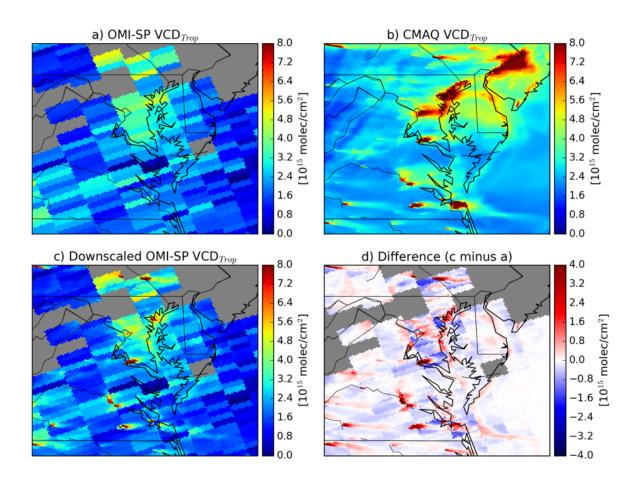
**Figure 5.** Tropospheric NO<sub>2</sub> VCD maps from (a) OMI SP, (b) CMAQ, and (c) downscaled OMI on July 29, 2011. The panel (d) shows the difference between downscaled and standard tropospheric NO<sub>2</sub> VCD data (c minus a). The gray areas represent pixels with effective cloud fraction > 0.3.
