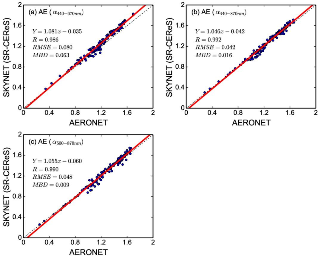
Figure 3: Comparison of SKYNET with AERONET Ångström exponent (within 1 minute) at 440–670 nm, 440–870 nm and 500–870 nm over Beijing. Only data with AOD > 0.4 are shown. The red solid line is the fitted linear regression curve.
