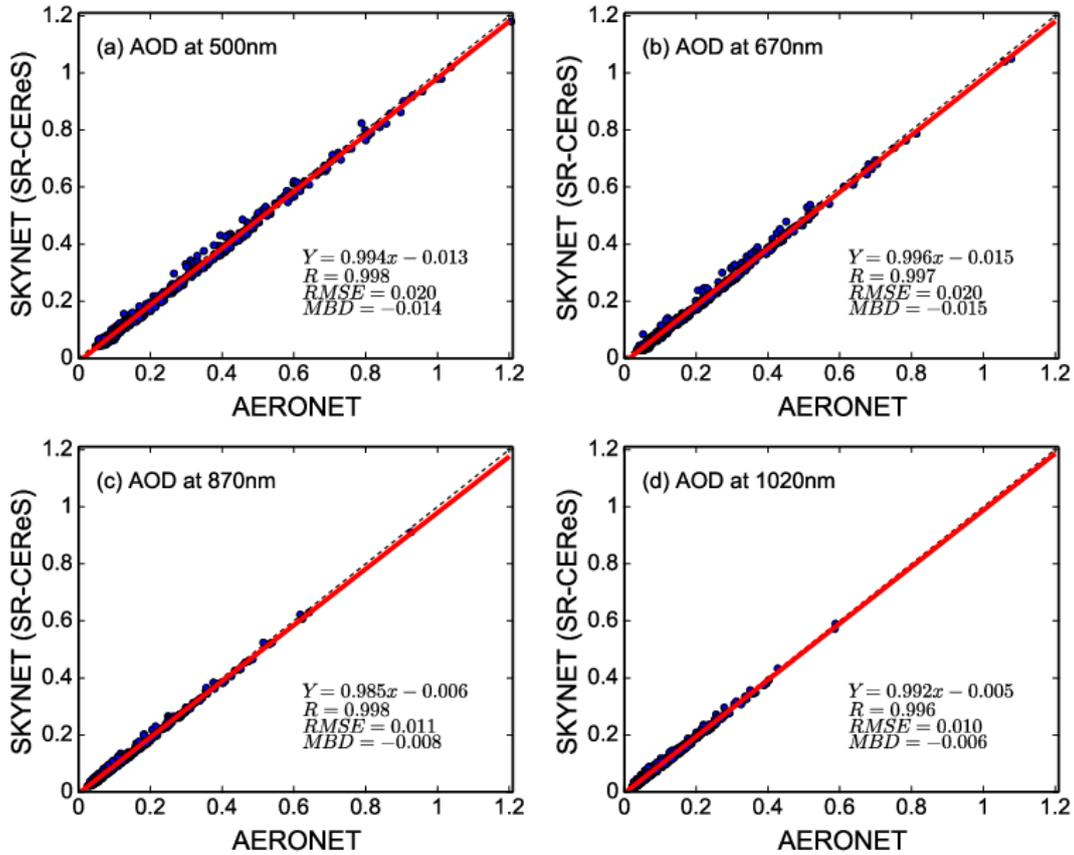
Figure 2: Comparison of SKYNET SR-CEReS-retrieved AOD with that from AERONET (within 1 minute) at 500, 670, 870 and 1020 nm over Beijing. The red solid line is the fitted linear regression curve.
