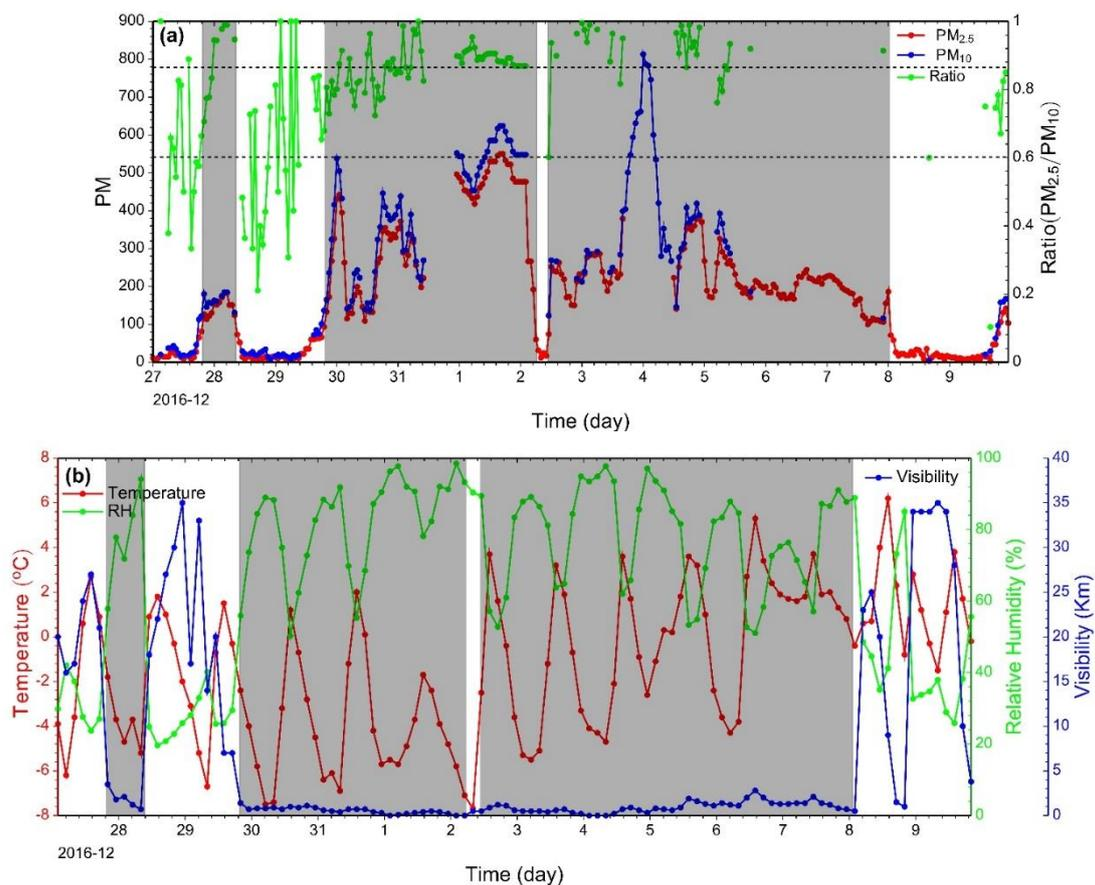
**Figure 10: Temporal variations of (a) PM<sub>2.5</sub>, PM<sub>10</sub>, and their ratio (PM<sub>2.5</sub>/PM<sub>10</sub>), and (b) meteorological data including temperature (°C), RH (%), and visibility (km), from 27 December 2016 to 9 January 2017. The shaded parts represent the pollution periods.**
