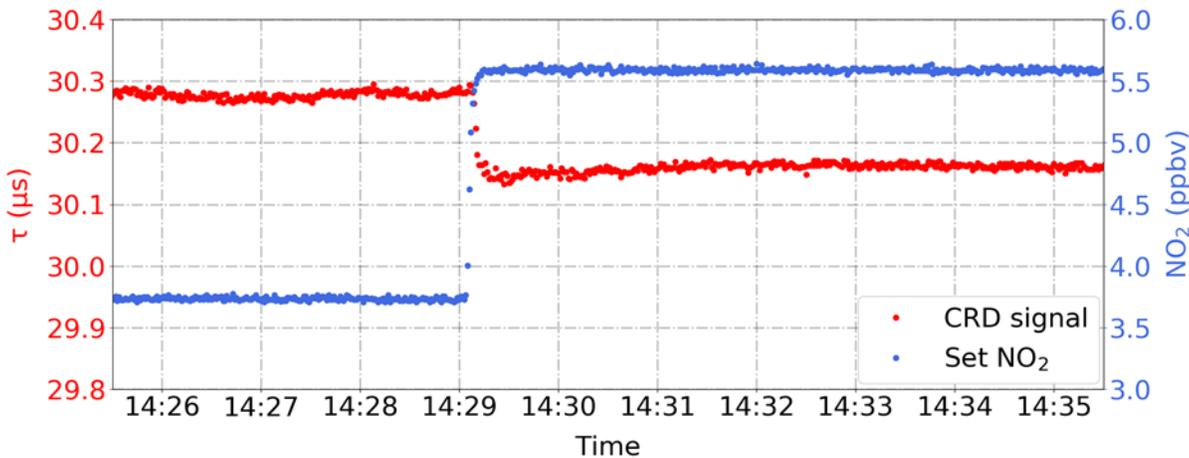
Figure RC1\_I: PerCEAS response to a step change in sampled  $\text{NO}_2$  mixing ratio
