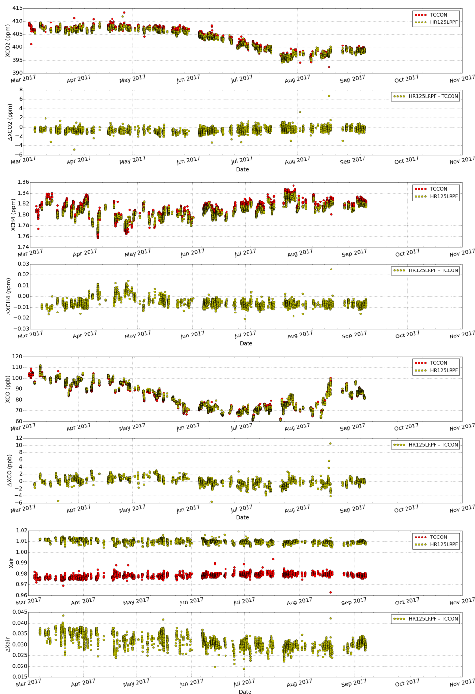
Figure 5. Timeseries of XCO 2 (first row panel), XCH 4 (third row panel), XCO (fifth row panel) and Xair (seventh row panel) retrievals for TCCON and HR125LR using the standard procedure using TCCON a priori for measurements performed at Sodankylä in 2017. The difference of XCO 2 (second row panel), XCH 4 (fourth row panel), XCO (sixth row panel) and Xair (eighth row panel) time series for HR125LR relative to the reference TCCON results.
