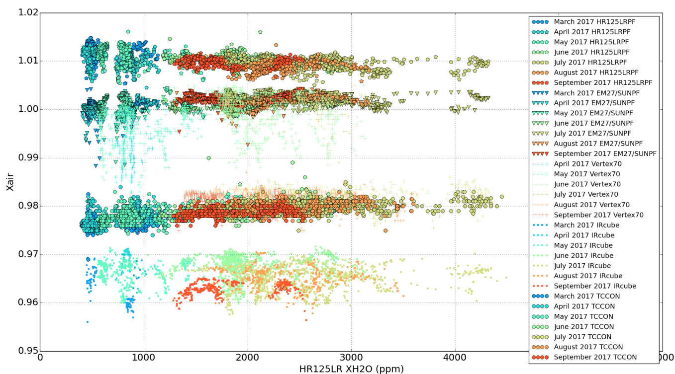
Figure 14. X_{air} plotted for HR125LR, EM27/SUN, Vertex70, IRcube and TCCON w.r.t. the total column water vapour retrieved by the reference HR125LR measurements. The colours represent the measurement performed during the different months of the year.
