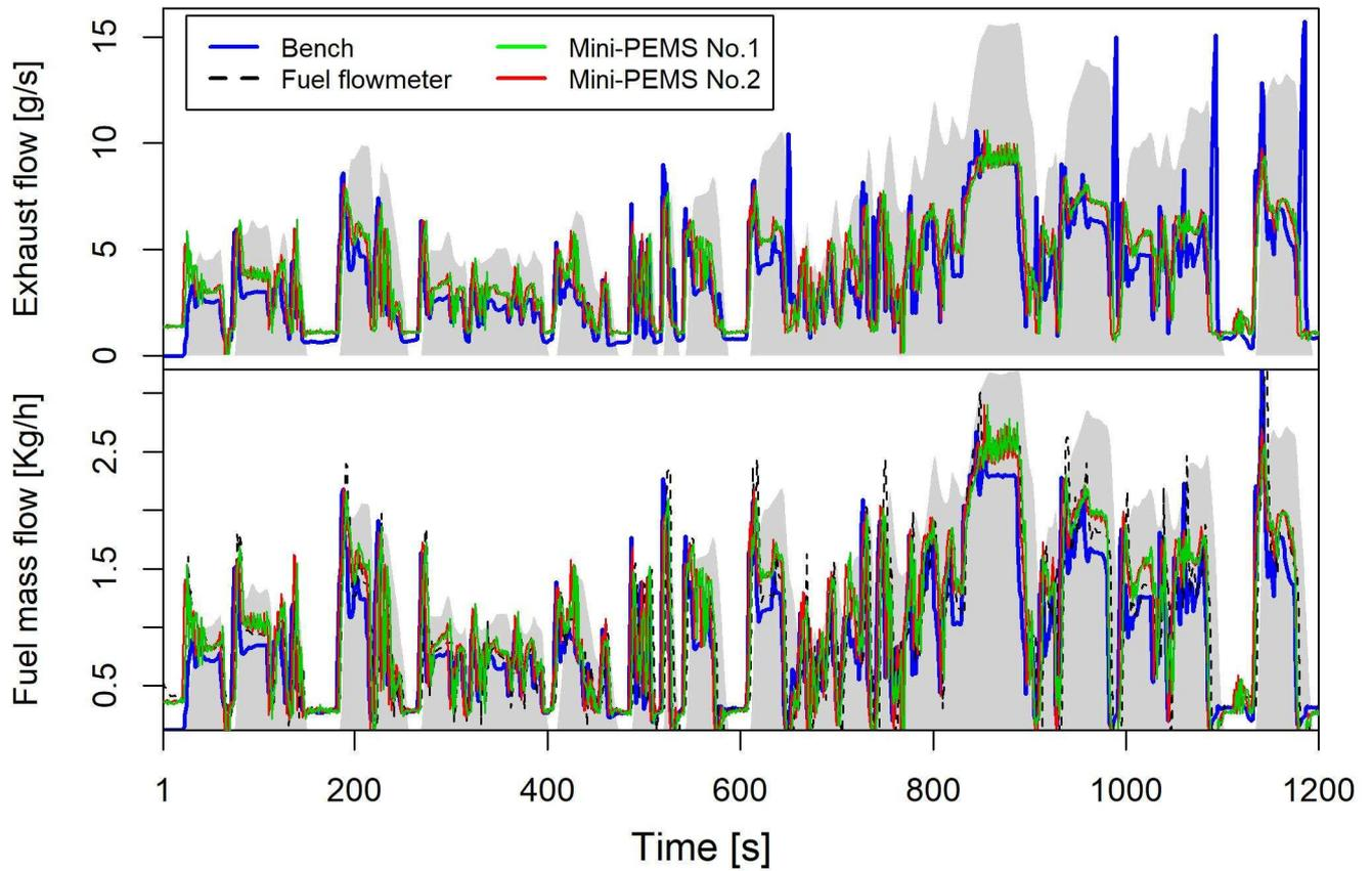
Figure 3. Upper panel: Comparison of the exhaust flow from bench instrumentation calculated with the CO<sub>2</sub> tracer method and from the 2 Mini-PEMS during Test 5. Lower panel: Comparison of fuel consumption (i) measured by a dedicated fuel flowmeter (KMA); (ii) calculated with the carbon balance method using HC, CO and CO<sub>2</sub> mass emissions rates from bench instrumentation; and (iii) calculated from Mini-PEMS No. 1 and No. 2.
