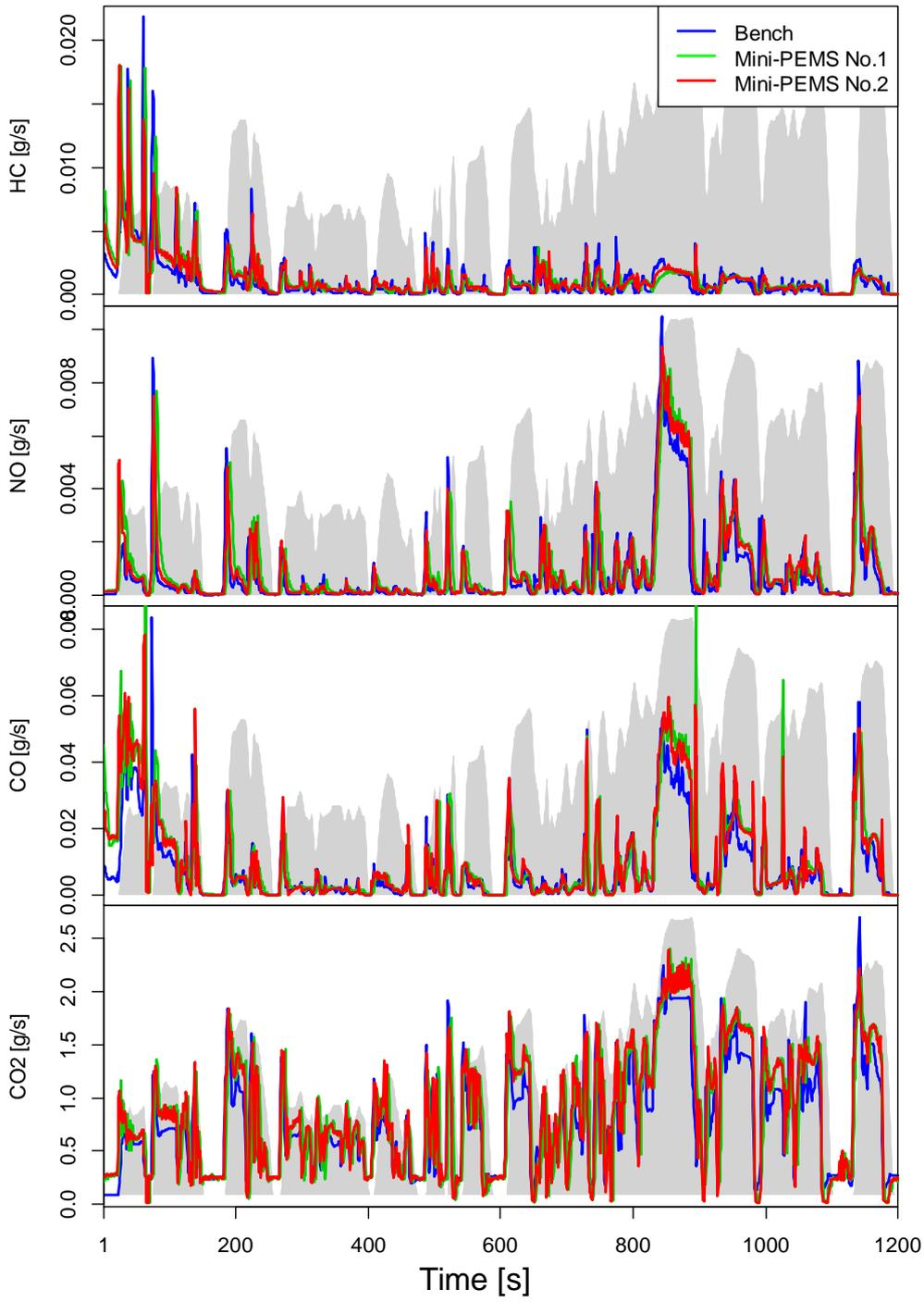
**Figure 4. Mass flow rates of HC, NOx, CO and CO<sub>2</sub> from bench instrumentation and from the two Mini-PEMS for Vehicle 2 during Test 5 (WMTC).**
