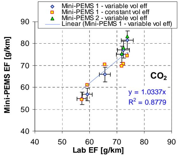
5 Figure 5. Emission factors of HC, NO<sub>x</sub>, CO and CO<sub>2</sub> from bench instrumentation (horizontal axis), and from Mini-PEMS No. 1 (vertical axis) obtained during roller bench tests. For Mini-PEMS no. 1, variable volumetric efficiency, error bars represent estimated known measurement uncertainty of 5% for Mini-PEMS and for laboratory, 3% for CO and CO<sub>2</sub>, 5% (10% for 50 mg/km) for HC, 7.5 mg/km for NO<sub>x</sub>.
