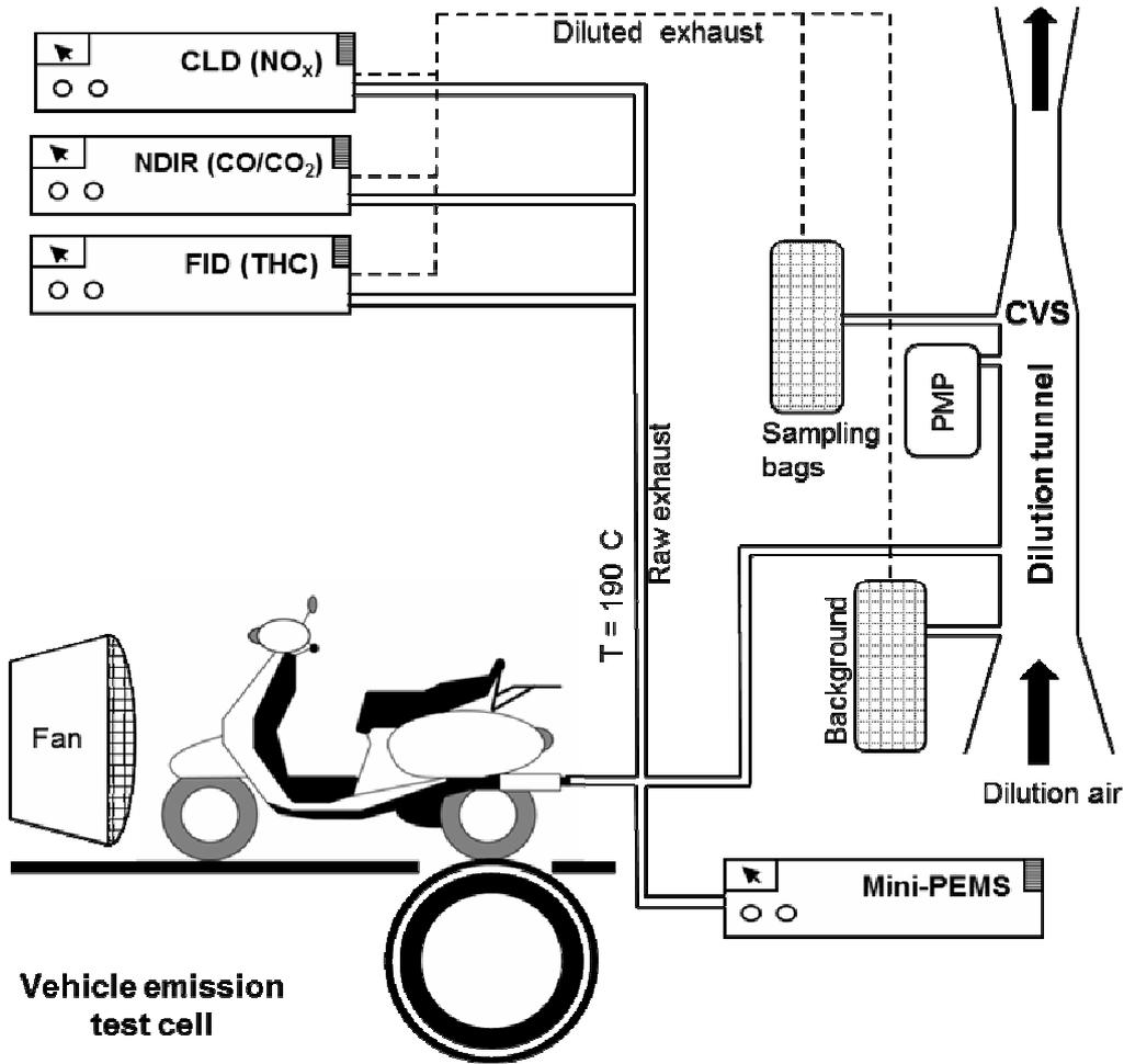
Figure 1. Schematic of the test cell and laboratory instrumentation. Exhaust emission measurements are performed at the tailpipe and after dilution through a constant volume sampler (flow rate  $\approx 5\text{m}^3/\text{min}$ ) by two independent gas analyzer systems. The Mini-PEMS collects part of the raw exhaust; see text for details.
