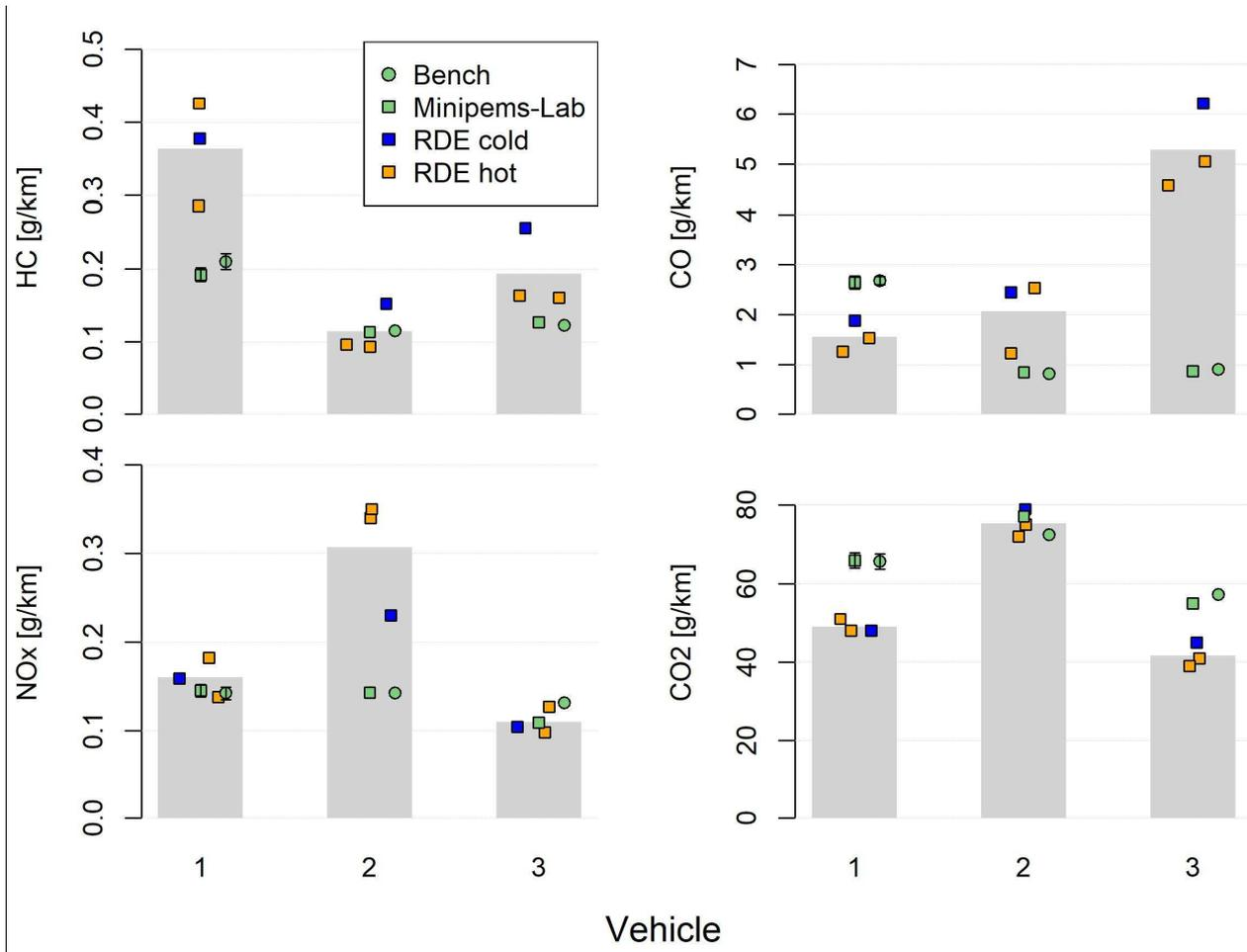
5 **Figure 7. Summary of real driving and laboratory emission factors. Roller bench emissions were obtained with laboratory instrumentation (green circles) and the Mini-PEMS (green squares). Grey bars are average real driving emission factors obtained with the Mini-PEMS from on-road cold start (blue squares) and hot start tests (orange squares). Error bars appear only on the first column in order to preserve readability.**
