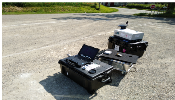
Fig. 7: The CHRIS spectrometer with the attached tracker during one of the 2018 MAGIC campaigns.
