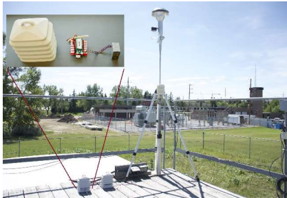
167 168 Figure 1: The low-cost sensor used in the study and the ambient inlet of the reference method – SHARP Model 5030
