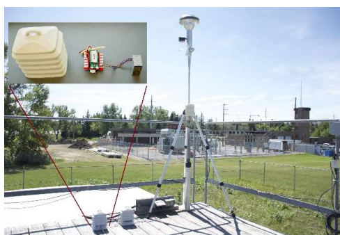
165 166 Figure 1: The low-cost sensor used in the study and the ambient inlet of the reference method – SHARP Model 5030
