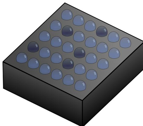
**Figure 1.** Schematic of a typical cold plate array, with droplets arranged in a grid on a heat sink. The heat sink is typically cooled by liquid Nitrogen or a Peltier device. The diagram shows some droplets frozen (dark).
