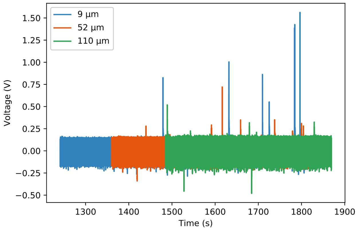
**Figure 3.** Sections of voltage time graphs for three different thicknesses of PVDF overlaid on top of each other. Each positive spike represents the freezing of a microlitre droplet of pure water. The offset at the start shows the similar noise amplitude for each thickness.
