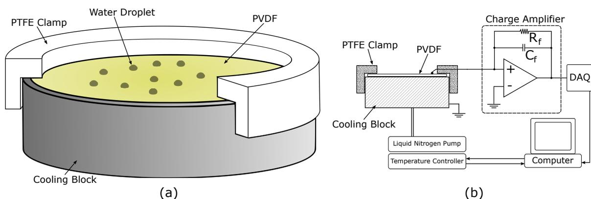
**Figure 2.** (a) A cut-away diagram of the cooling block with PVDF and clamp in place. The wire used to make contact with the upper surface is not shown. (b) A schematic of the experimental set-up including a simplified circuit diagram of the charge amplifier.
