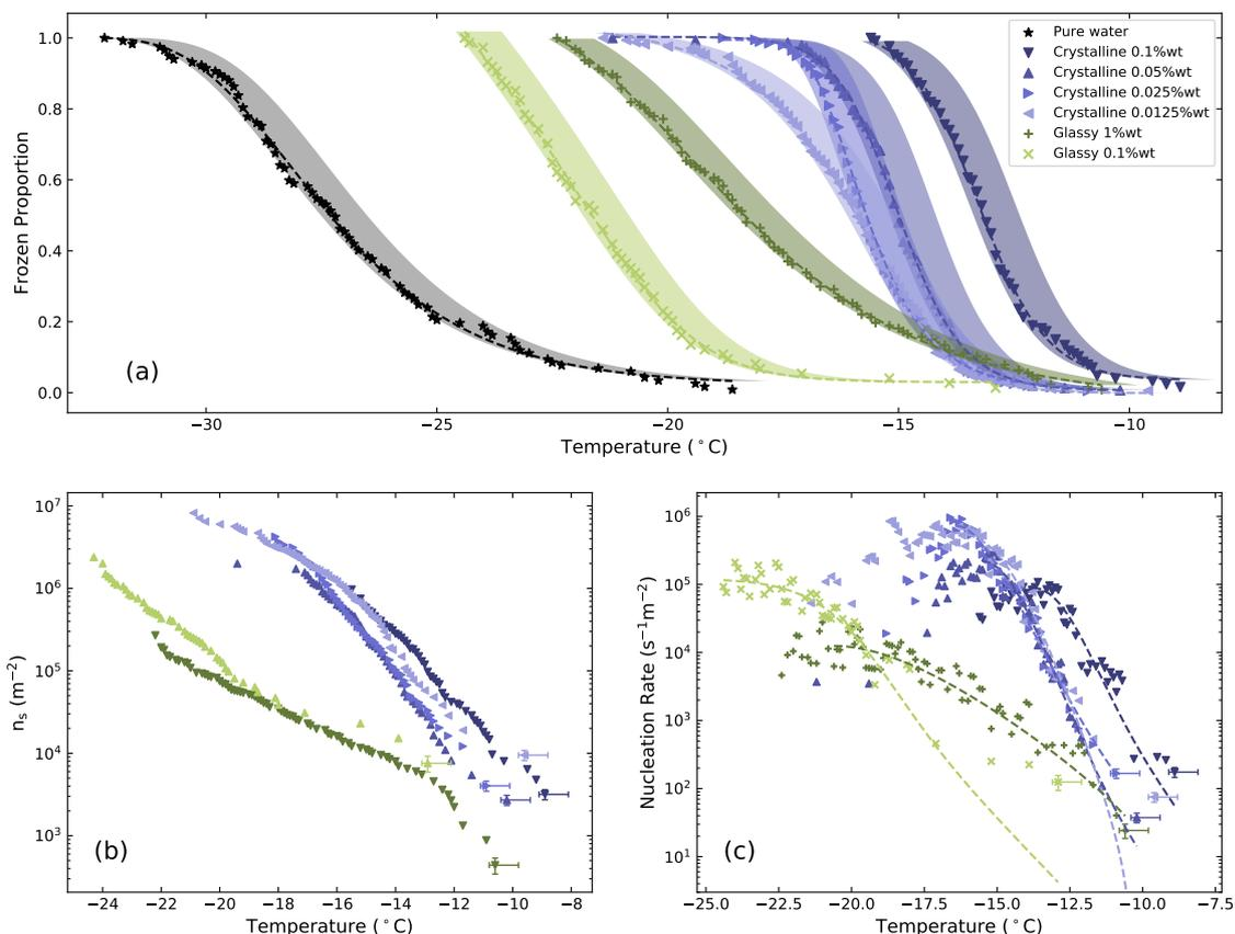
**Figure 5.** **a** Frozen fraction curves for 1  $\mu\text{l}$  droplets of water containing different fractions of glassy and crystalline K-Feldspar. The background freezing rate of the instrument is also shown as the pure water frozen fraction. **b** Ice nucleation active site density, normalised by the surface area present in each droplet. **c** The nucleation rate calculated from classical nucleation theory. Only the error bars of the first data point of each sample are shown for clarity.
