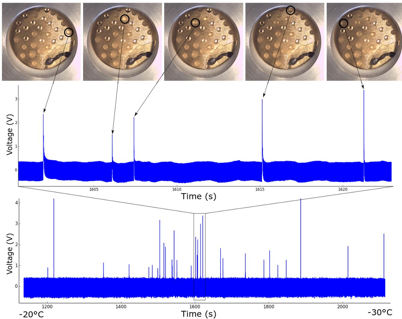
**Figure 4.** Raw data from a typical experimental run, in this case pure water droplets measured to determine the background freezing rate of the instrument. Each spike represents a droplet freezing, as shown in the upper graph and corresponding pictures. Approximate temperatures corresponding to the start and end of the run are shown at the bottom.
