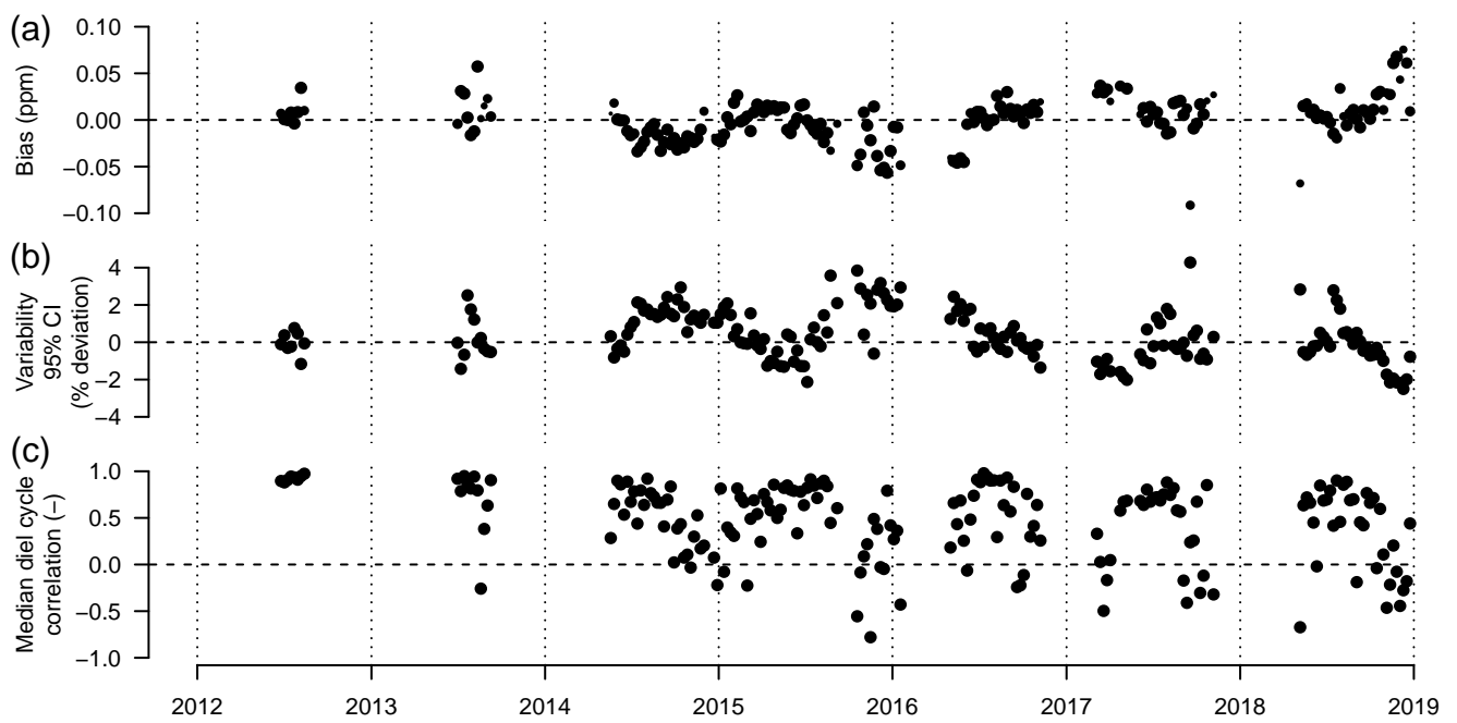
Figure 10. (a) Weekly median bias, (b) median variability, and (c) correlation between weekly median diel cycles of TGS 2600 sensor #1-1 and the reference. Symbol size is proportional to relative data coverage.
