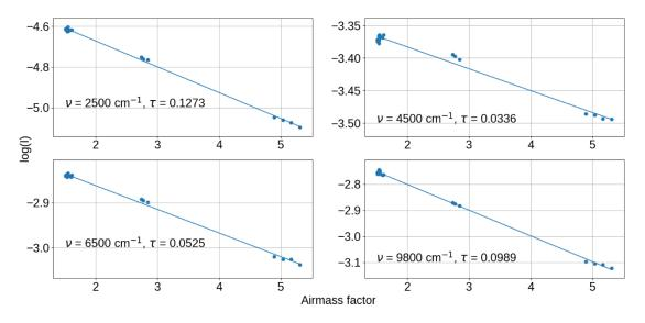
Figure 2: Langley plots from selected wavenumbers in the 4, 2.1, 1.6 and 1.02 μm atmospheric windows, along with the total optical depth obtained at that wavenumber. Taken from observations of 18 Sept 2008.
