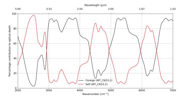
Figure 18: Proportion of the 18 September 2008 Camborne optical depth attributable to the self and foreign continua as calculated using the MT\_CKD3.2 model. The total optical depth is shown by the red line in Figure 7.
