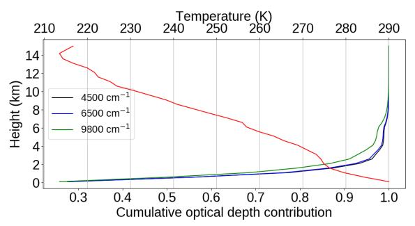
Figure 12: Fractional contribution to the total continuum optical depth (using MT\_CKD 3.2) with height from the surface up to 10 km at three wavenumbers. The temperature profile (top axis) derived from radiosonde on the 18 September 2008 is shown in red.
