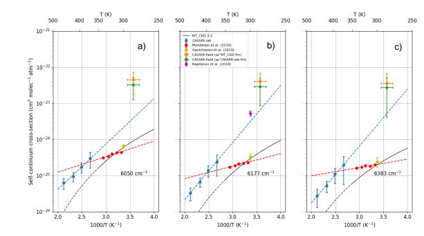
Figure 15: Self-continuum absorption cross-section against temperature for various datasets at (a) 6050, (b) 6177 and (c) 6383 cm<sup>-1</sup>. The error bars indicate the k = 1 uncertainties. Marker size is greater than the stated uncertainty where error bars not visible. The dashed black line indicates the region outside of the expected applicability of MT\_CKD. The dashed blue and red lines indicate extrapolations of the CAVIAR-lab and Grenoble temperature dependence respectively.
