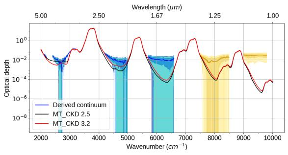
Figure 7: Langley-derived CAVIAR-field continuum optical depth and optical depth for two versions of the MT\_CKD water vapour continuum for 18 September 2008. The blue shaded regions indicate the k = 1 uncertainties, the cyan regions indicate the k = 2 uncertainties. The yellow shaded areas indicate spectral regions in which the CAVIAR-field derived continuum is potentially spurious and should be treated with caution (see Section 2).
