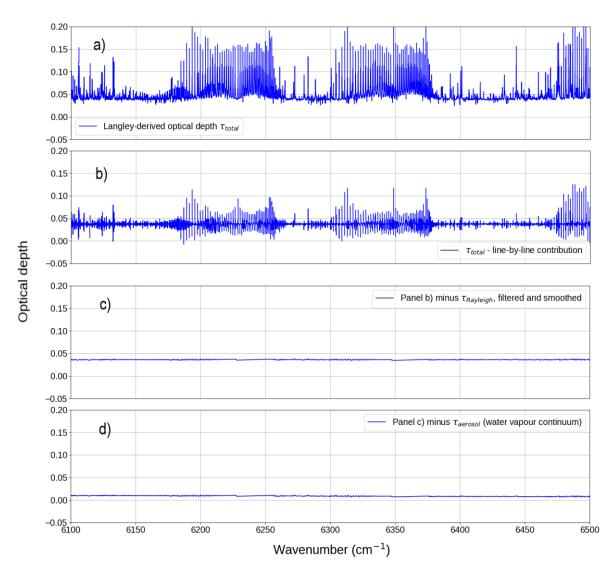
Figure 3: Example derivation of the water vapour continuum optical depth  $\tau_{cont}$  from the total optical depth  $\tau_{total}$  (a) via subtraction of  $\tau_{H20\_lines}$  and  $\tau_{other\_gases}$  (b), smoothing and subtraction of Rayleigh scattering  $\tau_{Rayleigh}$  and continuum absorption by other gases  $\tau_{other}$ (c), and finally subtracting  $\tau_{aerosol}$  to get the water vapour continuum optical depth (d).
