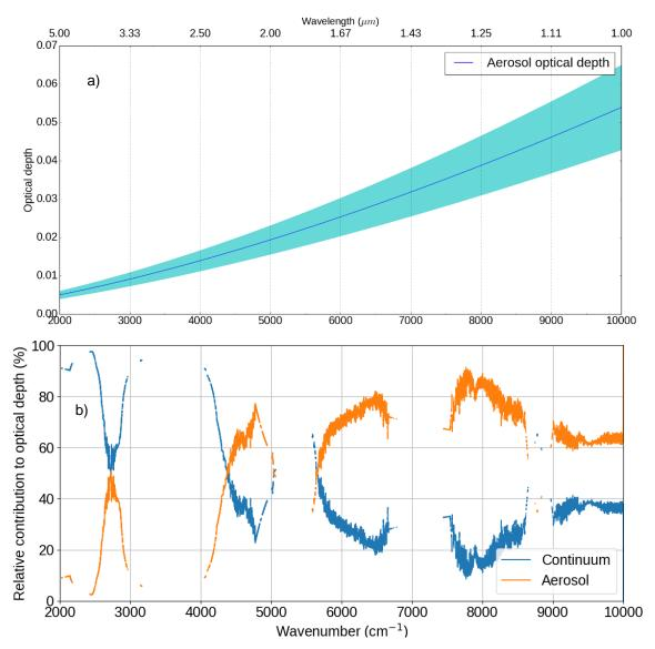
Figure 5: Panel a): Aerosol optical depth obtained from the Mie scattering calculations for 18 September 2008 with the Microtops  $\tau_{aerosol}$  at 1  $\mu m$ , along with the estimated k=1 uncertainties (shaded region). Panel b): Relative contribution of the continuum and aerosol in each of the near-infrared windows to the combination of the two ( $\tau_{aerosol} + \tau_{continuum}$ ).
