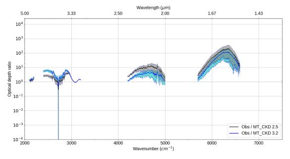
Figure 10: Ratio of Langley-derived CAVIAR-field continuum optical depth divided by MT\_CKD optical depth (for two different versions of MT\_CKD) in the 2.1 and 1.6 μm atmospheric windows for 18 September 2008. Uncertainties (shaded regions) shown at
