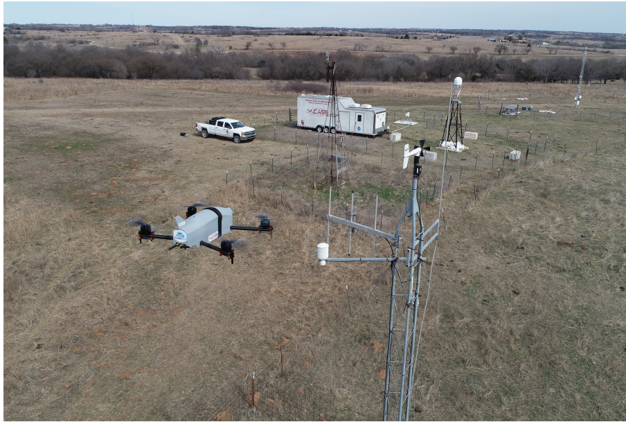
Figure 8. Picture of the CopterSonde hovering and tracking the wind next to the Oklahoma Mesonet tower at KAEFS. The aerial photo was taken by a DJI Phantom 4 Pro drone from above.
